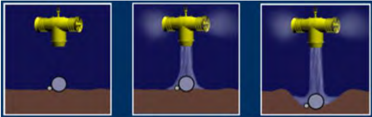
Figure 46 Mass flow excavation
