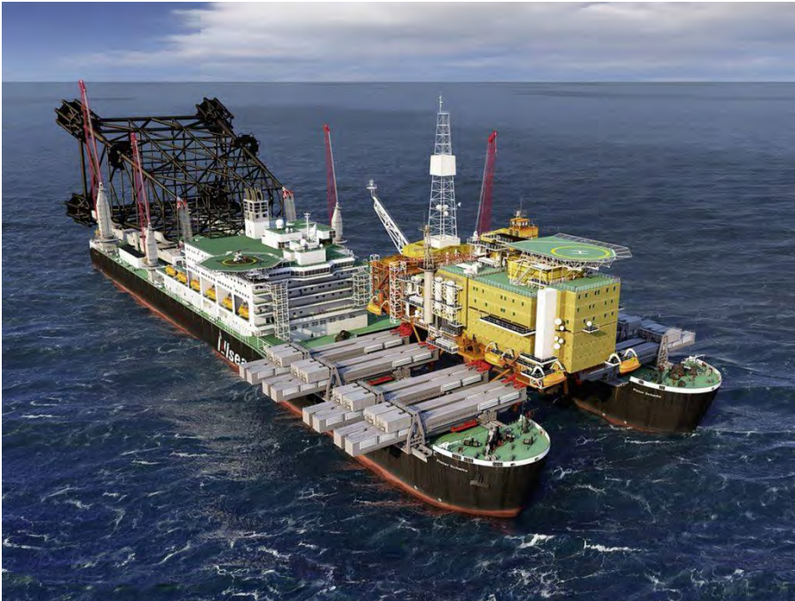
Figure 7c Catamaran installation with the Pioneering Spirit [source: allseas.com]
