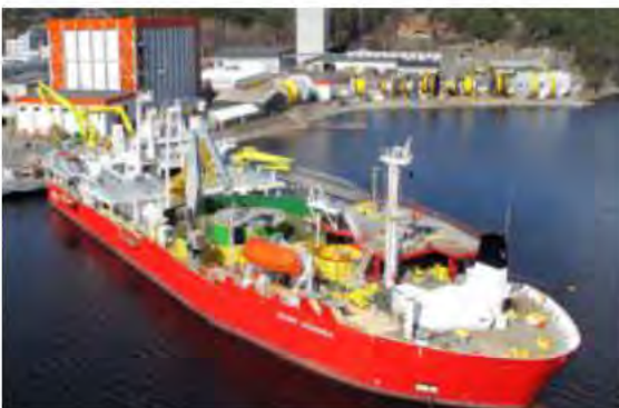
Figure 38 Typical deep water cable installation vessels
