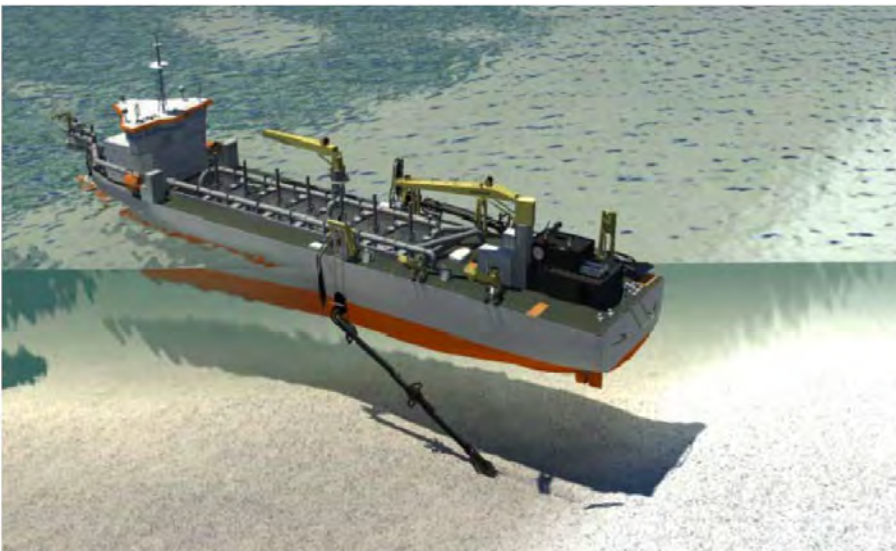
Figure 55 Trailing Suction Hopper Dredger
