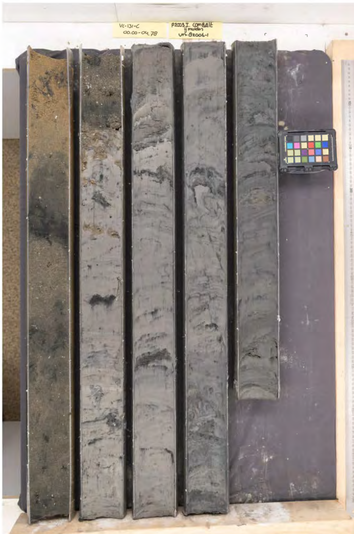
Figure 10. Clay sequence above 'Top of layered sediments' reflector
