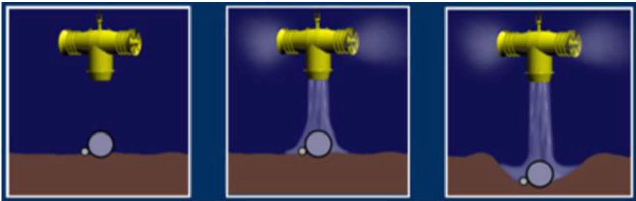
Figure 46 Mass flow excavation
