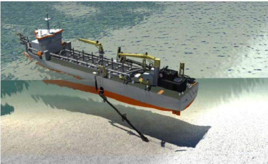
Figure 55 Trailing Suction Hopper Dredger
