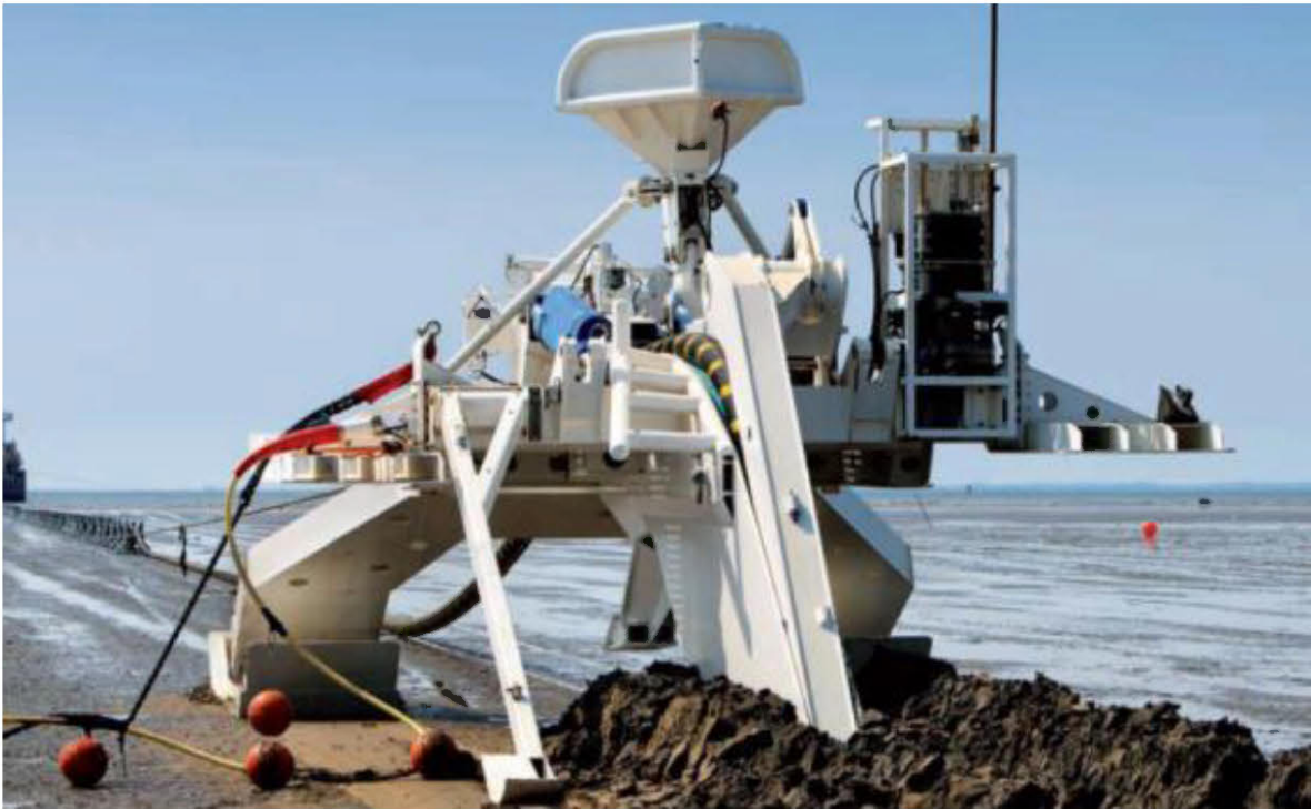
Figure 45 Sea Stallion cable plough
