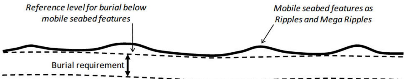
Figure 11 level for cable burial below ripples and mega ripples
