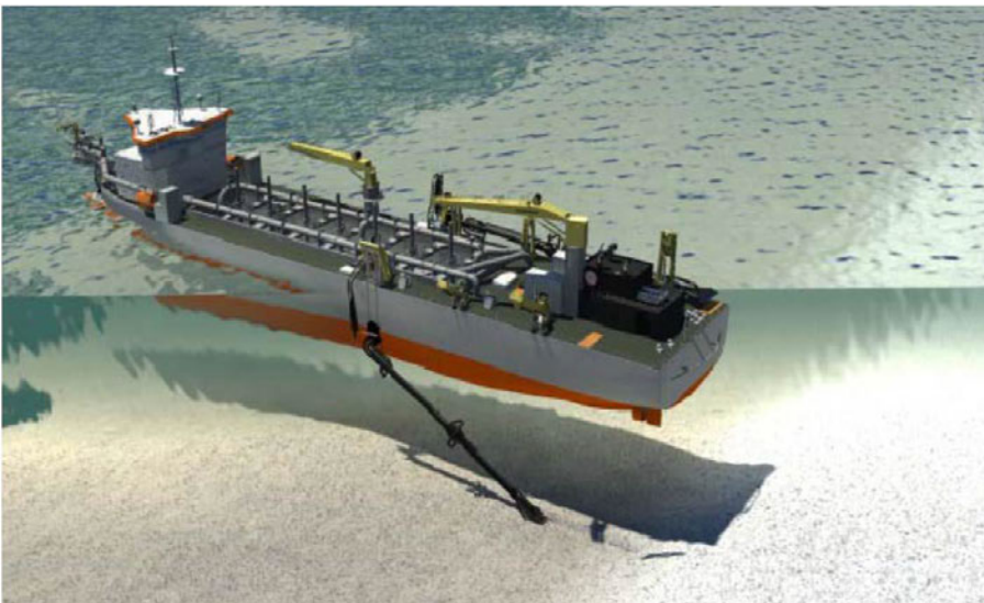
Figure 55 Trailing Suction Hopper Dredger
