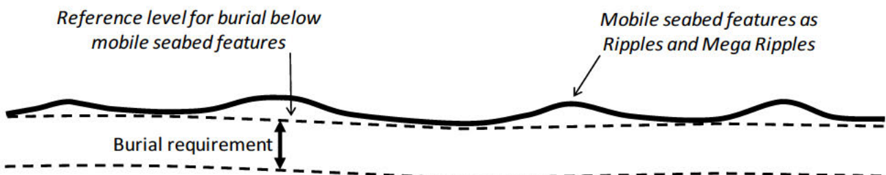
Figure 11 level for cable burial below ripples and mega ripples
