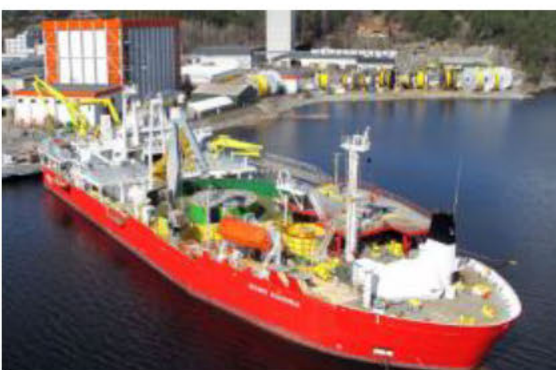
Figure 38 Typical deep water cable installation vessels
