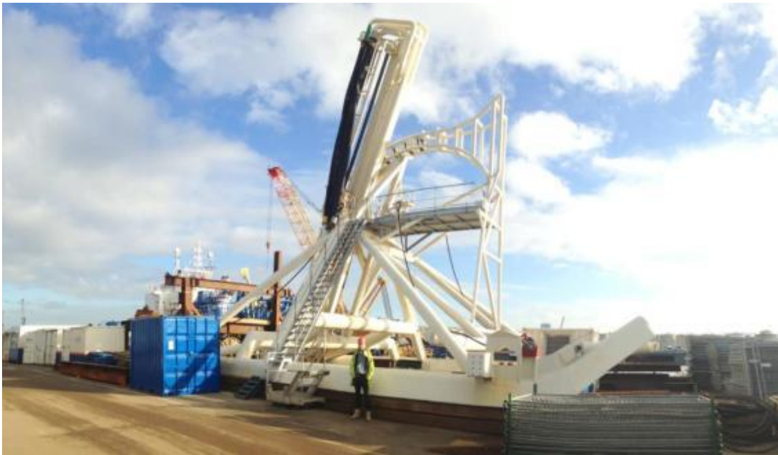
Figure 40 BSS2 jet sledge
