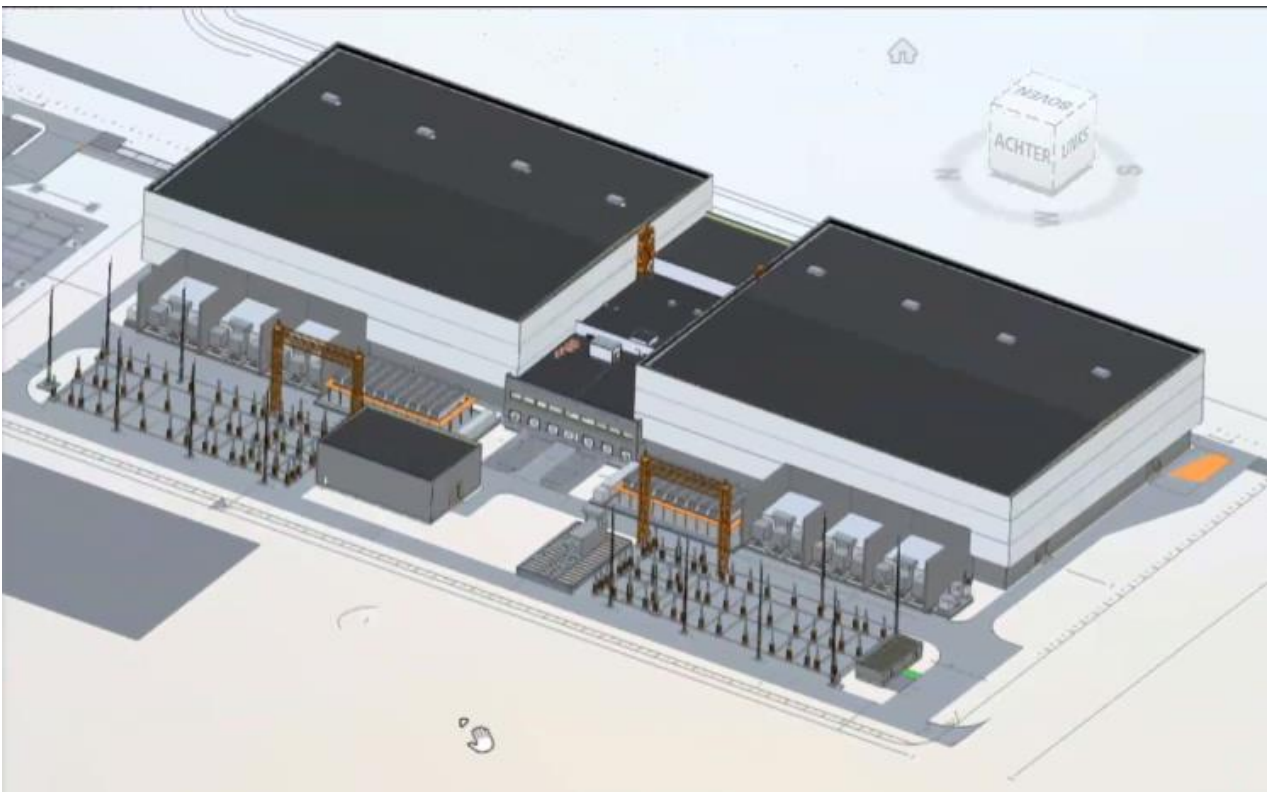
Figure 59 – 3D model onshore converter station Nederwiek
