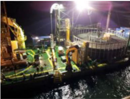
Figure 48 Typical nearshore cable lay barges
