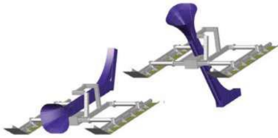
Figure 39 Typical Jet sledge
