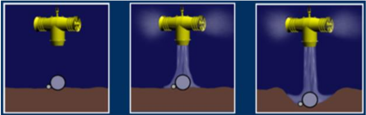
Figure 46 Mass flow excavation
