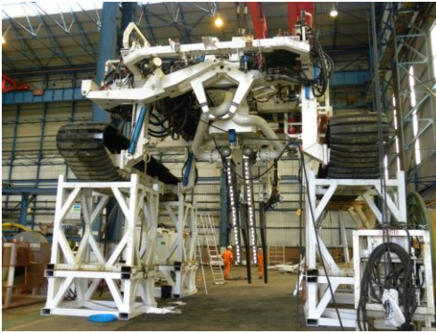
Figure 42 Typical ROV Jet trencher
