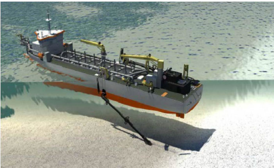
Figure 55 Trailing Suction Hopper Dredger
