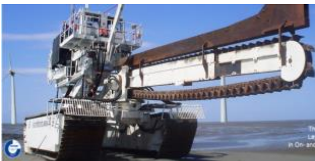
Figure 43 Typical Chain cutter
