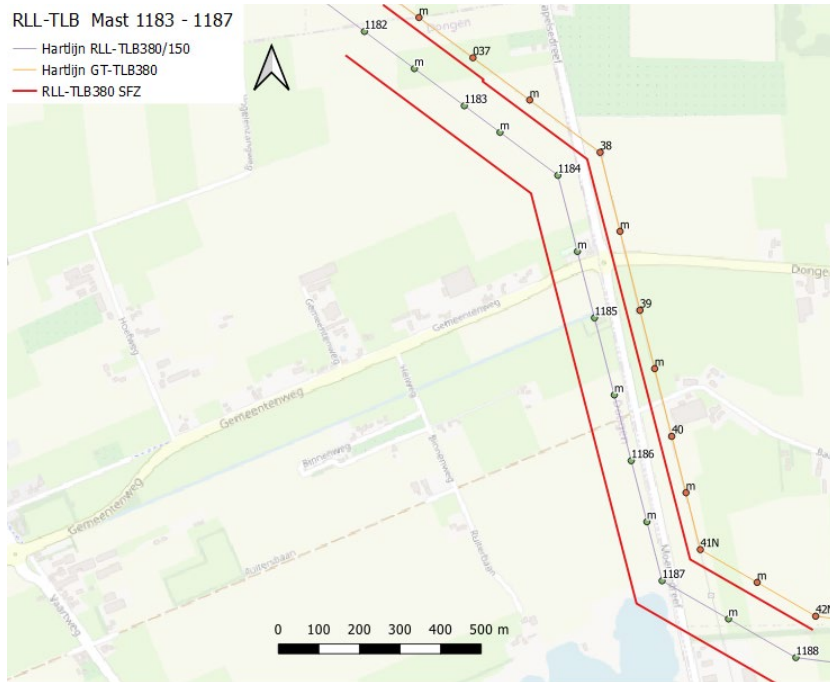
Figure 3-1 Overview of the rounded off SFZ between towers 1182 to 1188 of high voltage RLL-TLB380 without cumulative influence of nearby lines as per H1.4 product.
