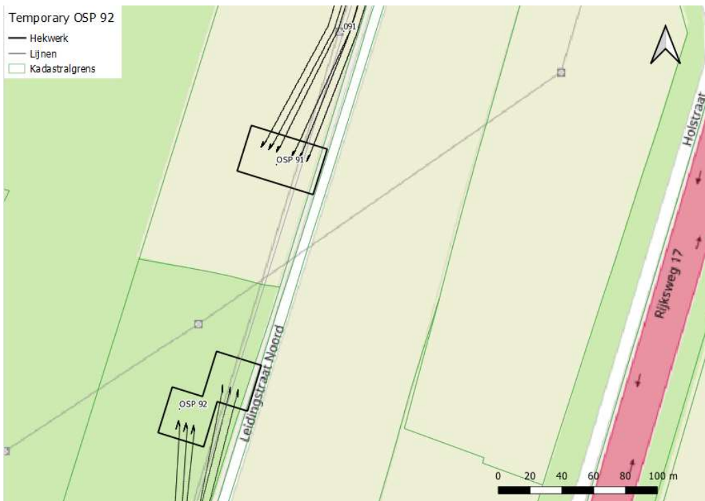
Figure 3-17 RSD-MDK150 Mast 92 (D+0) span to temporary OSP in QGIS view
