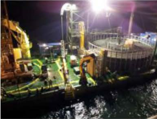
Figure 46 Typical nearshore cable lay barges
