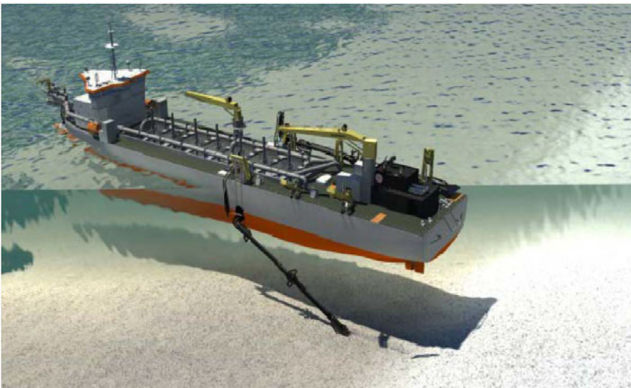
Figure 53 Trailing Suction Hopper Dredger
