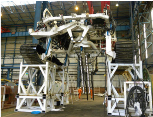
Figure 40 Typical ROV Jet trencher
