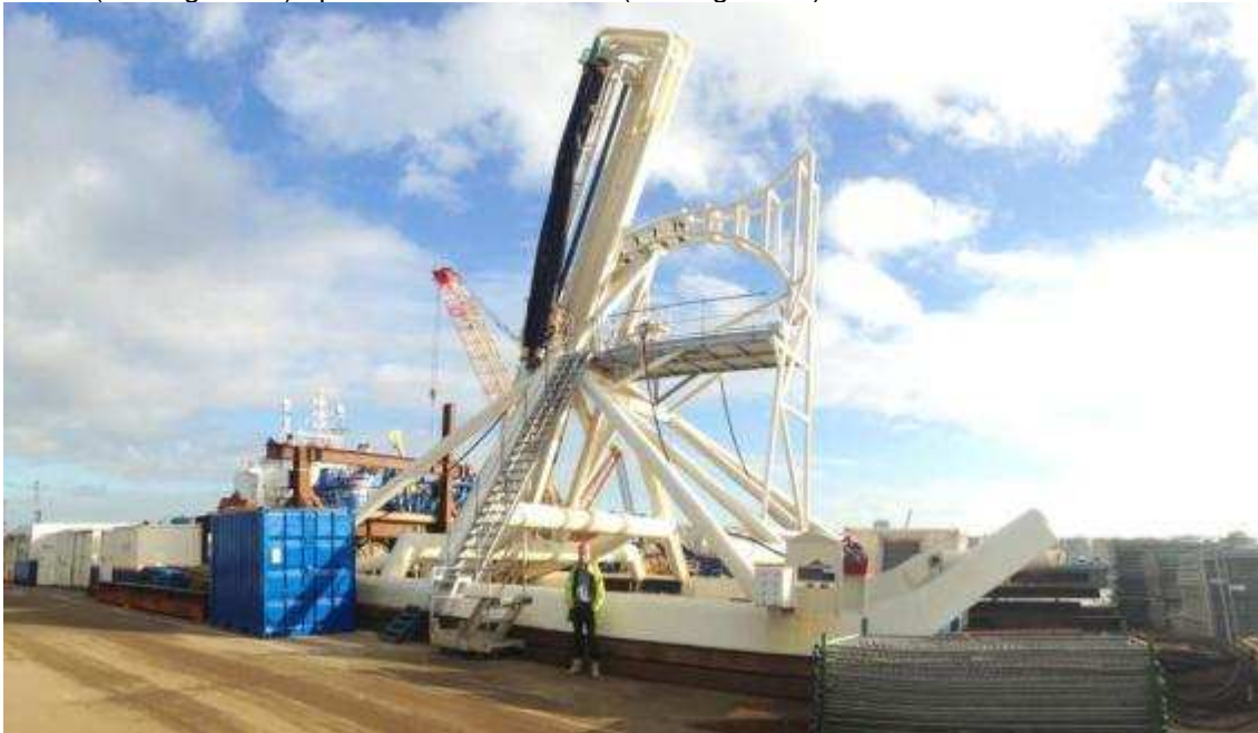
Figure 38 BSS2 jet sledge
