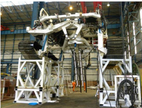
Figure 39 Typical ROV Jet trencher
