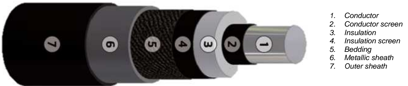
Figure 6 Typical HVAC 220 kV land export cable
