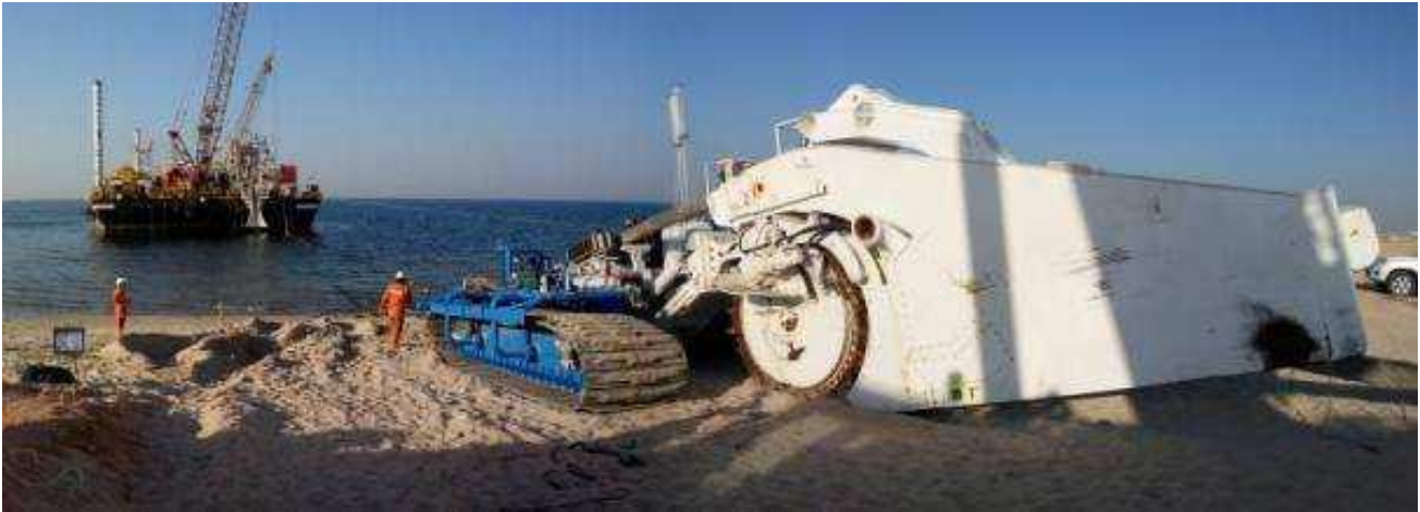
Figure 41 TM04 Wheel cutter cable trencher
