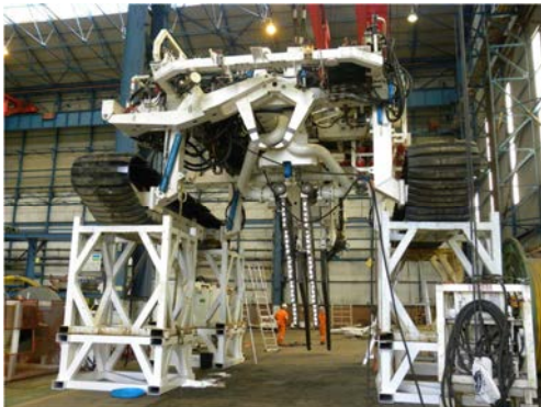
Figure 39 Typical ROV Jet trencher
