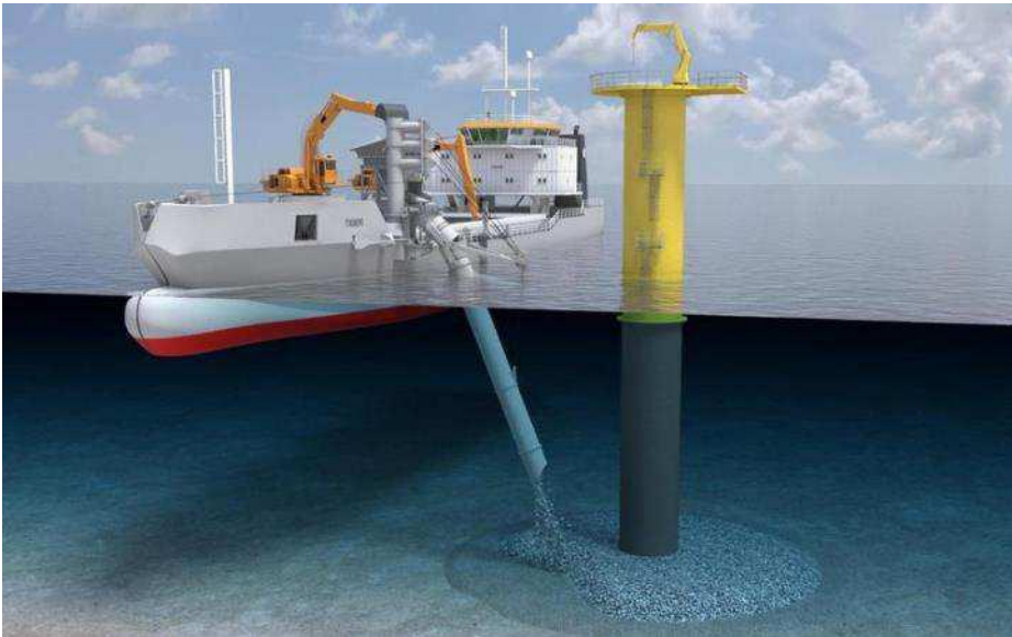
Figure 57 Rock installation vessel
