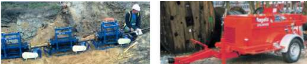
Figure 17 Typical cable tensioners (left) & cable winch (right)
