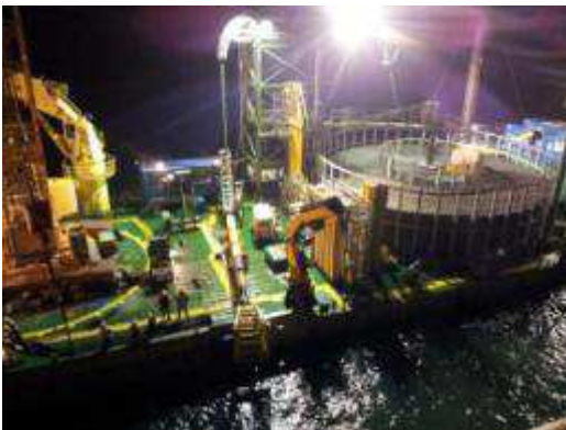
Figure 45 Typical nearshore cable lay barges
