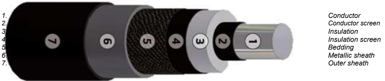
Figure 6 Typical HVAC 220 kV land export cable
