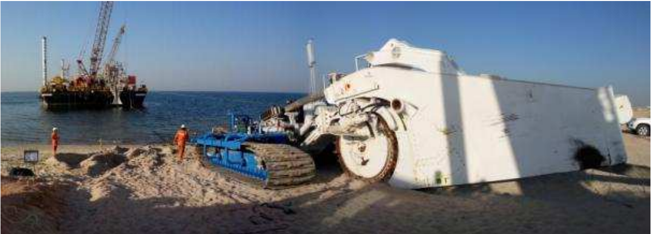
Figure 41 TM04 Wheel cutter cable trencher
