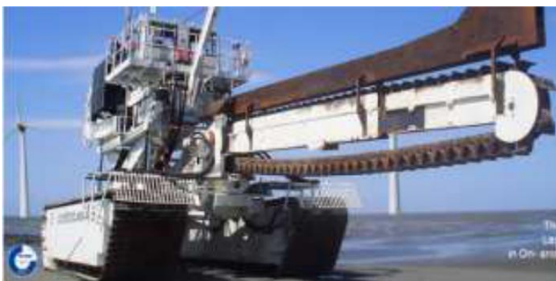
Figure 40 Typical Chain cutter
