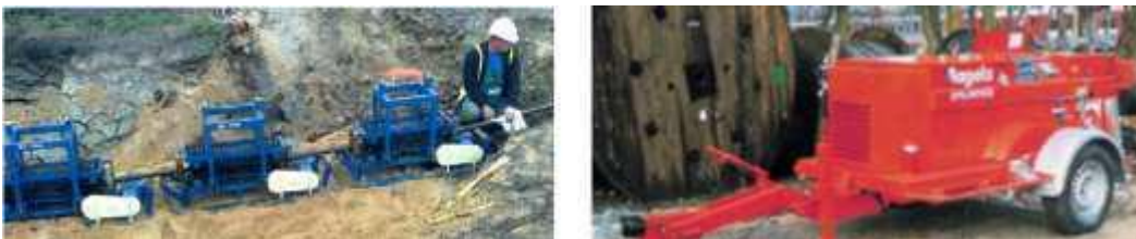
Figure 17 Typical cable tensioners (left) & cable winch (right)
