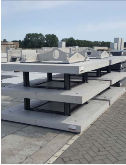
Figure 2. Squared terraced broodstock structure used in the pilot in offshore wind park Borssele V (Van Rie, 2020).
