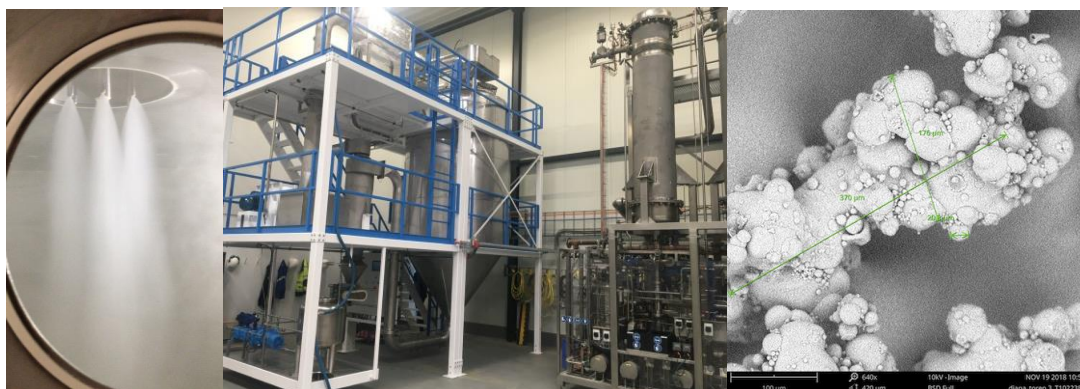
Figure 2; spray pattern in normal dairy agglomeration spray dryer. DW-1000 spray drier for small productions (SDW). Typical agglomerated powder
