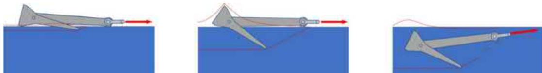
Figure 5.1: Left: Phase 1, shallow sliding and scratching at a speed larger than v_1 Middle: Phase 2, fluke penetration at nominal capacity at speeds between v_1 and v_2 Right: Phase 3, full penetration at nominal and better capacity at speeds below v_2
