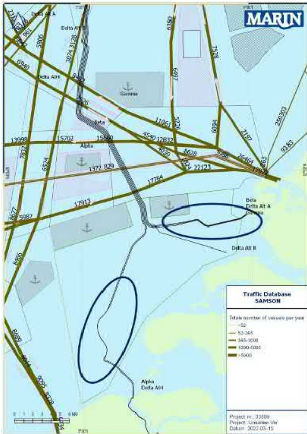
Figure 3-3 Indications of the parts of the trajectory related to stranding of vessels.
