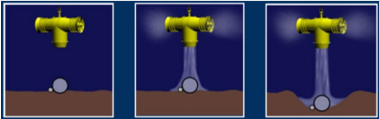
Figure 44 Mass flow excavation
