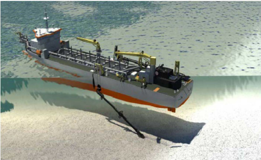
Figure 53 Trailing Suction Hopper Dredger
