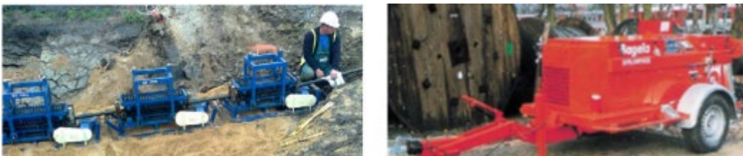
Figure 16 Typical cable tensioners (left) & cable winch (right)
