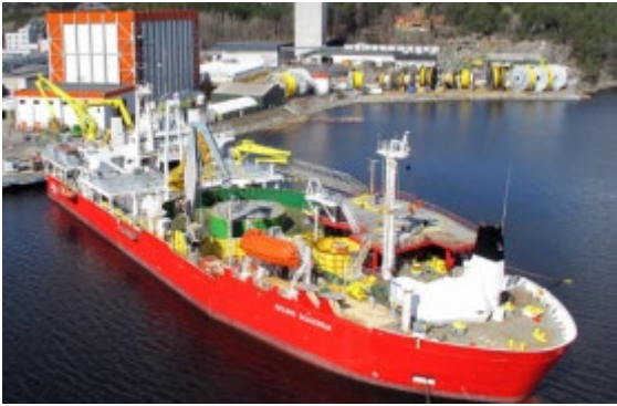
Figure 36 Typical deep water cable installation vessels
