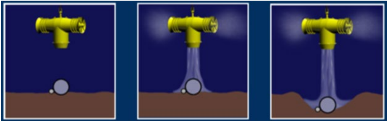
Figure 44 Mass flow excavation
