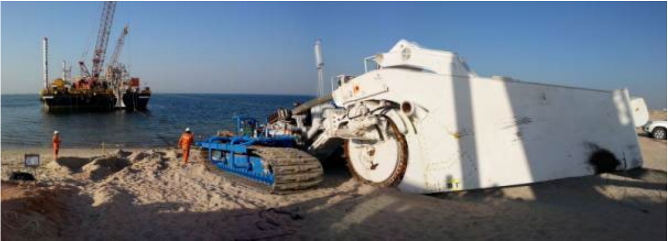
Figure 42 TM04 Wheel cutter cable trencher
