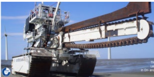
Figure 41 Typical Chain cutter
