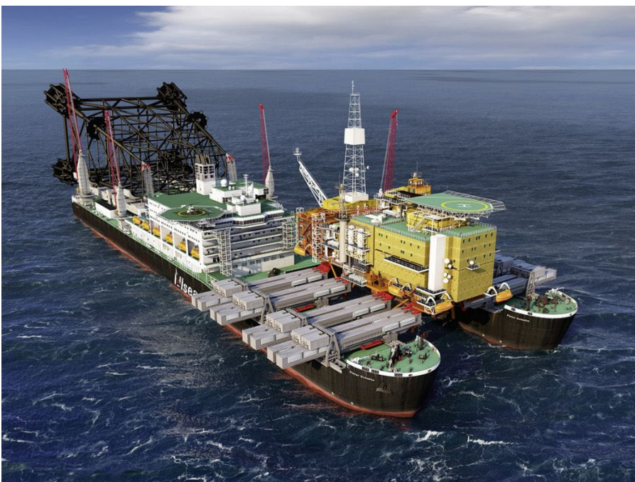
Figure 7b Catamaran installation with the Pioneering Spirit [source: allseas.com]
