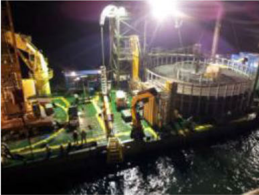
Figure 46 Typical nearshore cable lay barges
