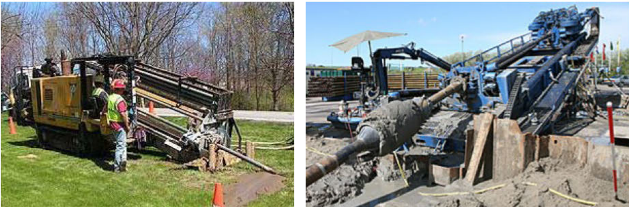
Figure 30 Example HDD rigs - [left] midi rig - [right] maxi rig
