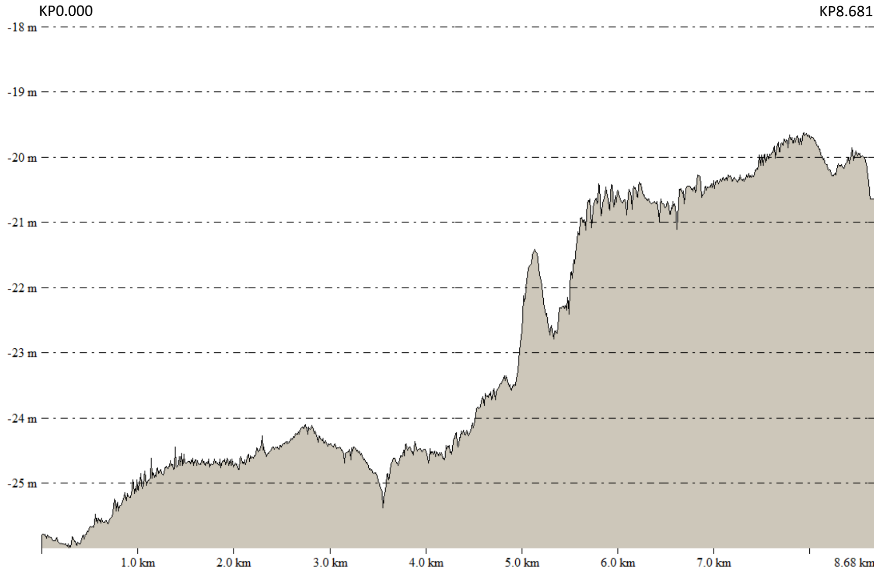
Figure 3: Bathymetric profile along the proposed cable route N5A Platform to Riffgat
