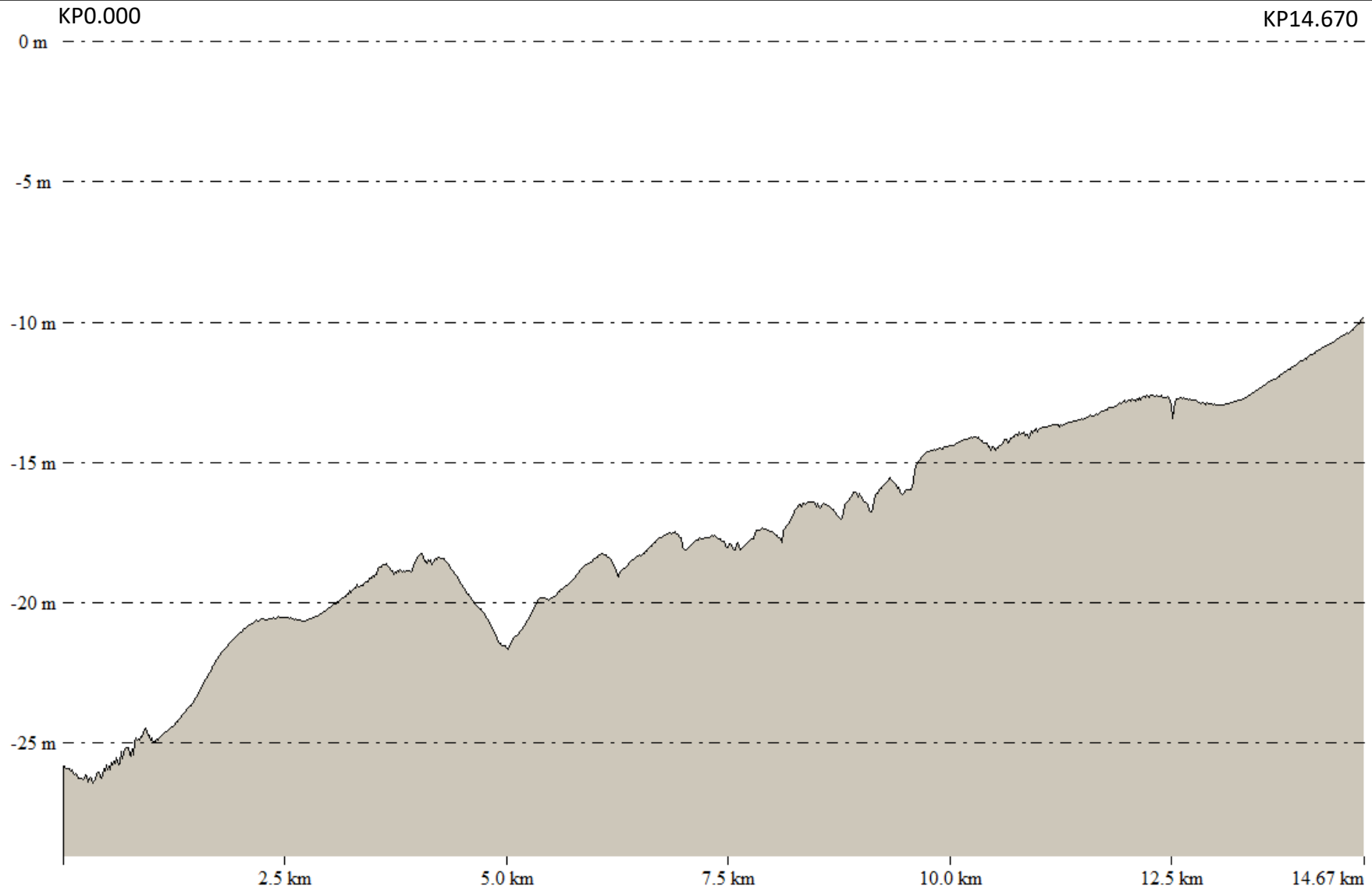
Figure 3: Bathymetric profile along the proposed pipeline route N5A to NGT Hot tap
