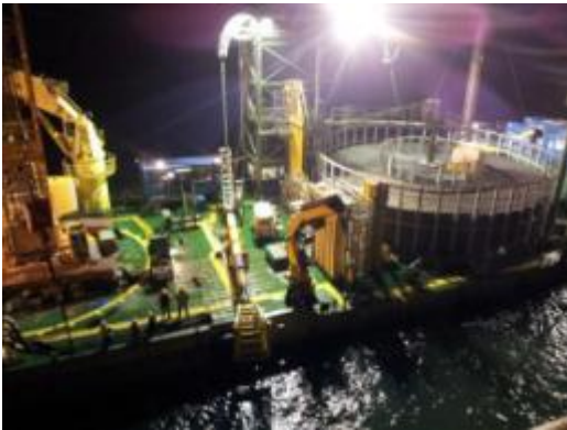
Figure 48 Typical nearshore cable lay barges
