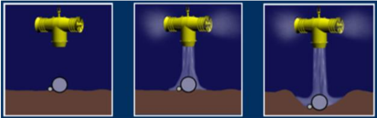
Figure 46 Mass flow excavation
