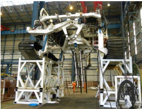
Figure 42 Typical ROV Jet trencher
