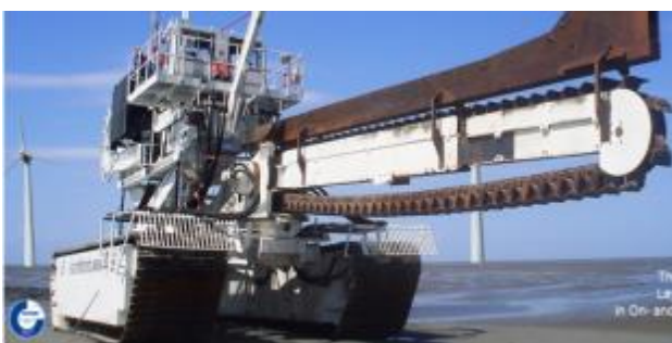
Figure 43 Typical Chain cutter
