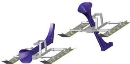
Figure 39 Typical Jet sledge
