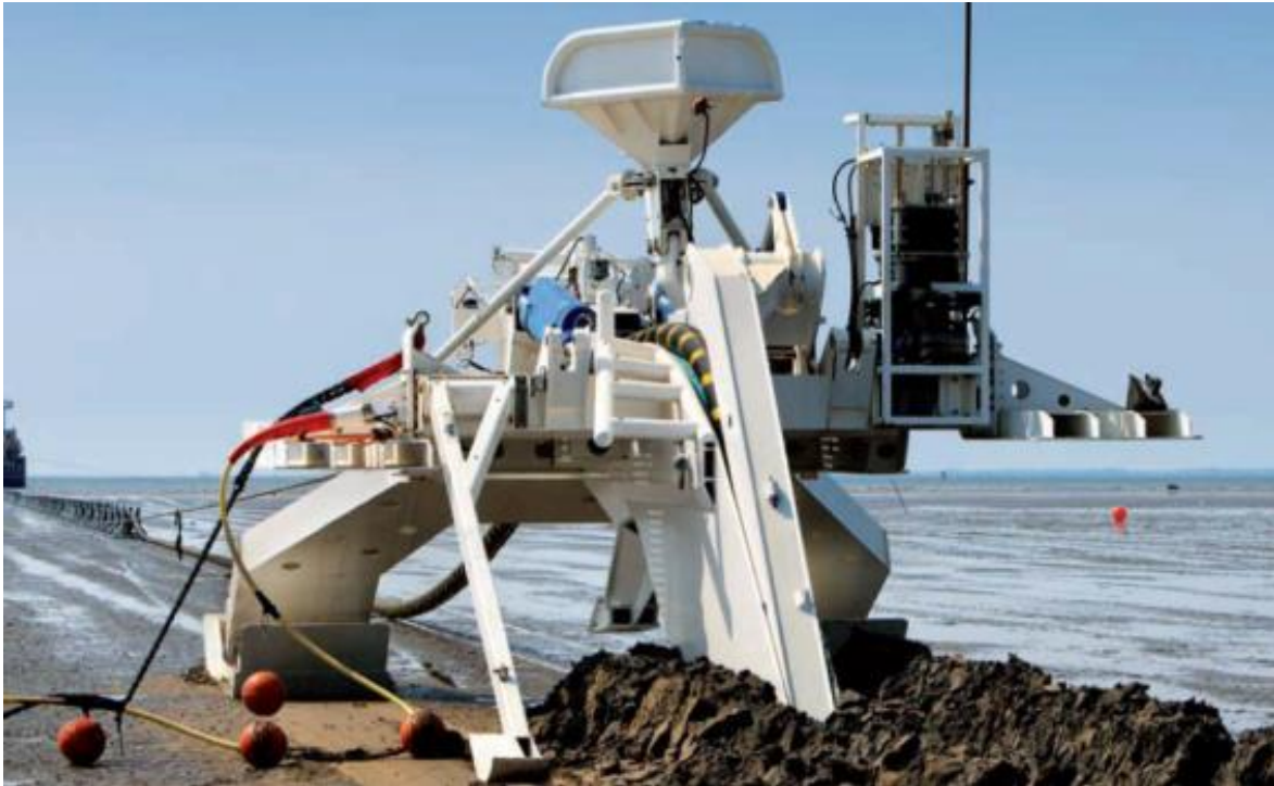
Figure 45 Sea Stallion cable plough
