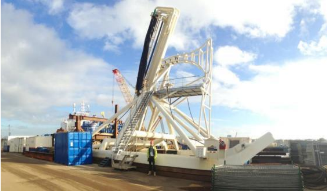
Figure 40 BSS2 jet sledge
