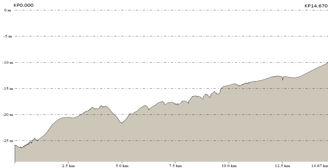
Figure 4-3 Seabed profile along pipeline route from N05-A Platform to NGT side tap connection
