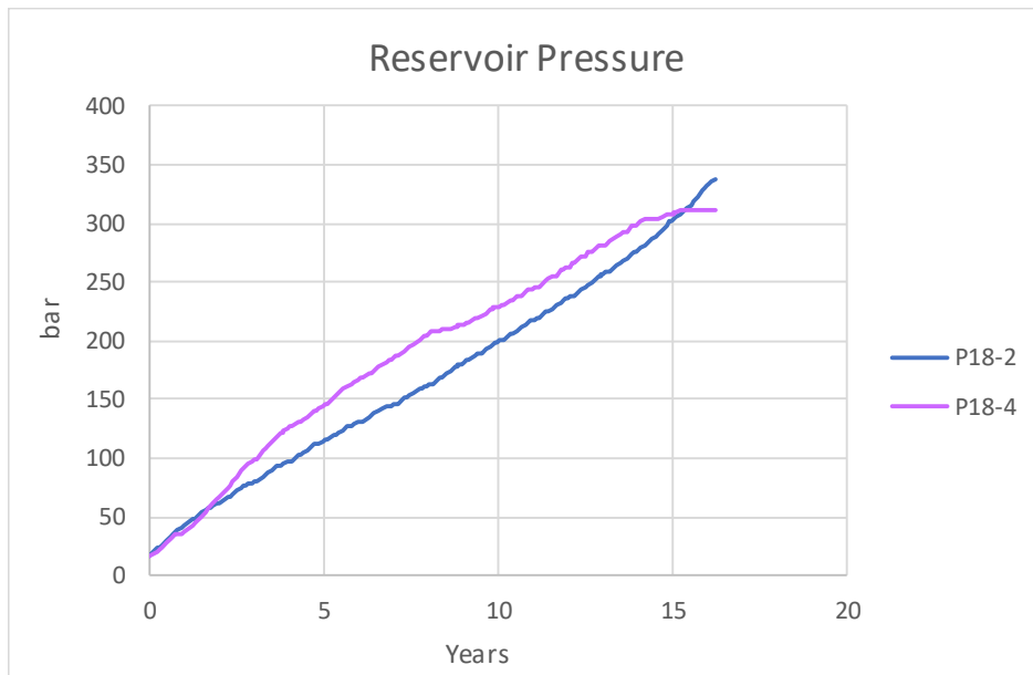
Figure 15: Reservoir pressure over time – commercial case (total 37.5Mt)
