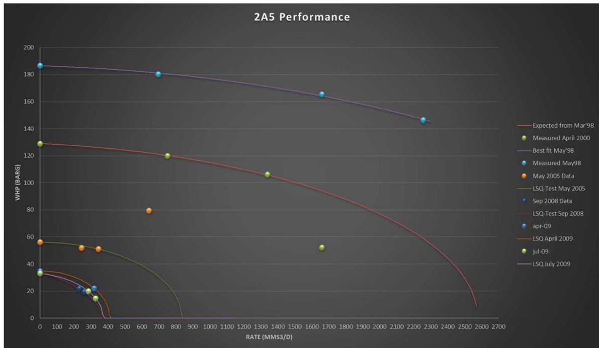
Fig. 15. IPR's constructed from the multi-rate tests for P18-2A5. THP-Q data from 1998 is compared to data from 2000 where a clear well performance degradation is observed
