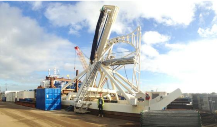
Figure 23 BSS2 jet sledge
