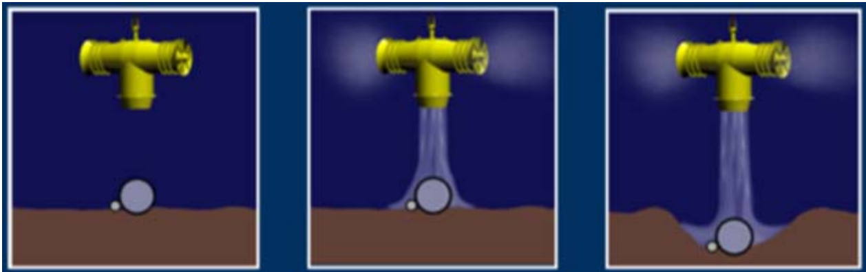
Figure 31 Mass flow excavation
