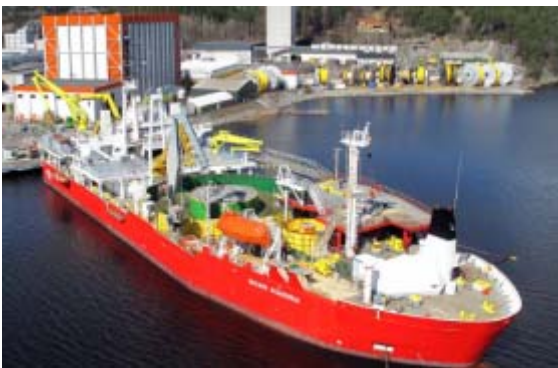
Figure 17 Typical deep water cable installation vessels
