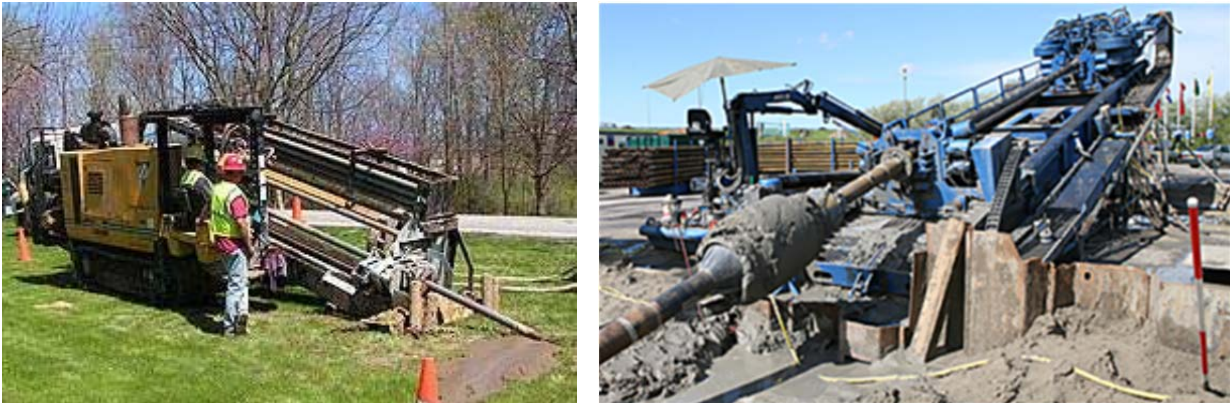
Figure 47 Example HDD rigs - [left] midi rig - [right] maxi rig
