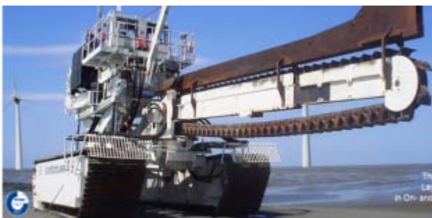
Figure 26 Typical Chain cutter
