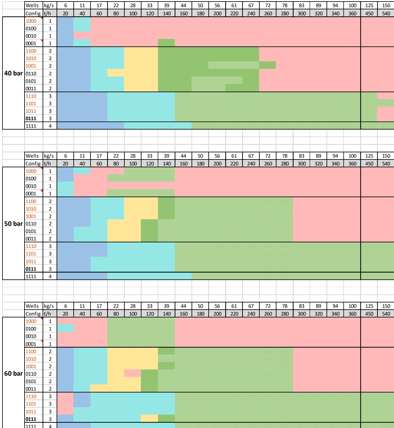
Figure 10: Operating envelope (of normal temperatures) for Pres 40bar to 60bar. (Although this also indicates the gas mode, Dense phase mode is indicated where both would be possible.)
