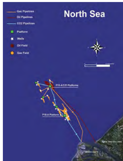
Figure 8.10: Location P15/P18 complex relative to the Dutch shore. Source: CO 2 offshore storage, deep under the Dutch North Sea, (image courtesy TAQA; TAQA, 2009)
