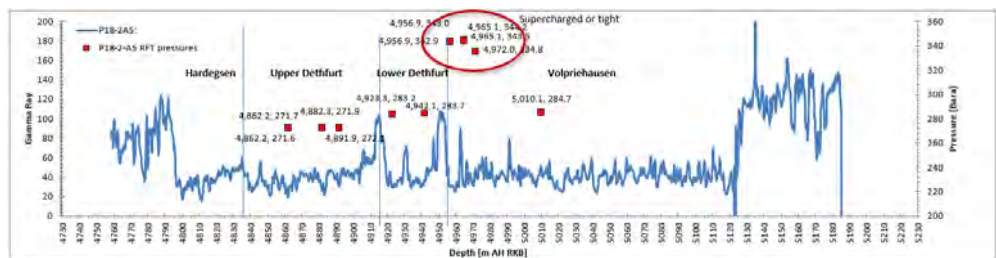
Figure 17-15: RFT measurements in Well P18-A5ST1 (red squares) showing differential depletion. Average pressure in the Upper Detfurth Fm is 272 Bara, in the Lower Detfurth Fm 283.5 Bara, and 284.7 Bara in the Volpriehausen Fm. Encircled points are either supercharged or tight.
