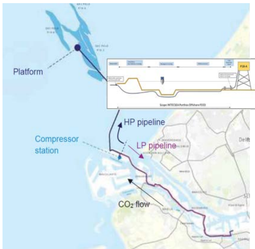
Figure 3: Overview of the Porthos CCS transport system.
