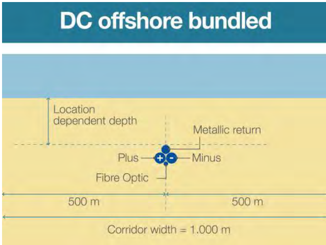
Figure 35a Cable corridor offshore section with bundled and touching cables
