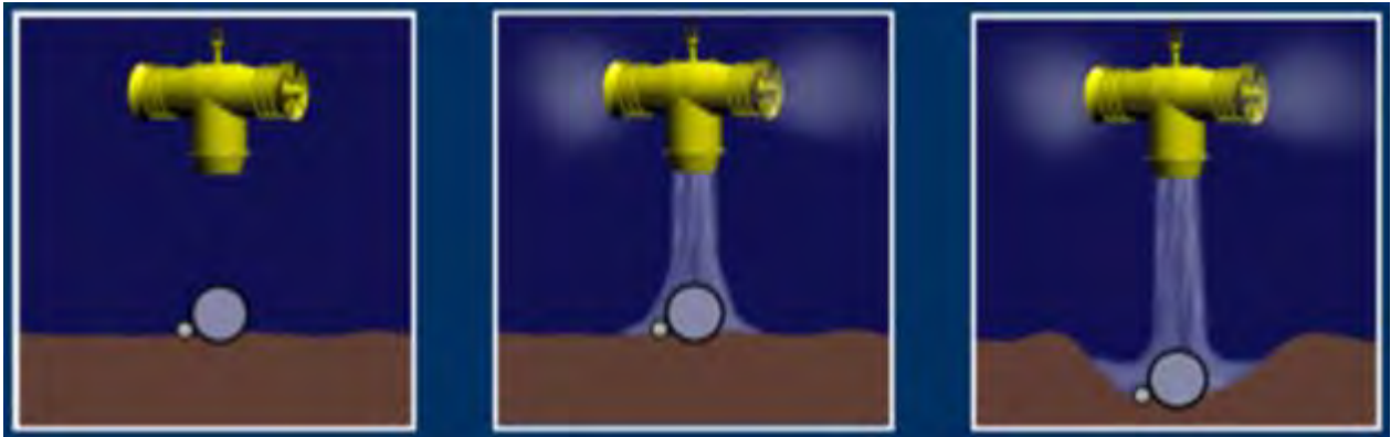
Figure 46 Mass flow excavation
