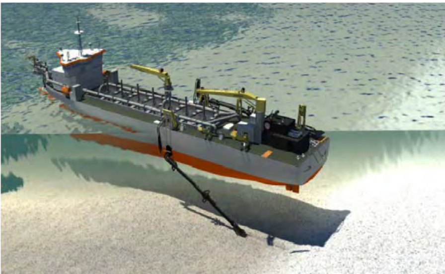
Figure 55 Trailing Suction Hopper Dredger
