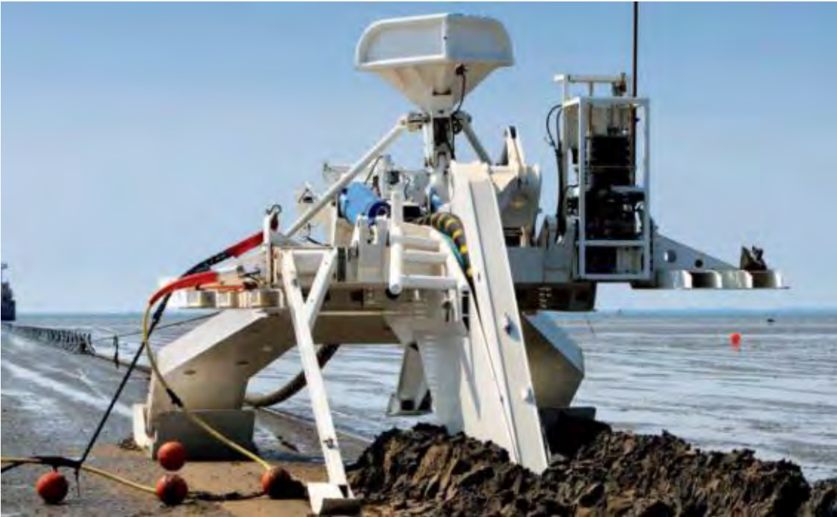
Figure 45 Sea Stallion cable plough
