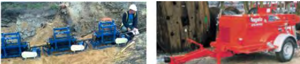
Figure 18 Typical cable tensioners (left) & cable winch (right)
