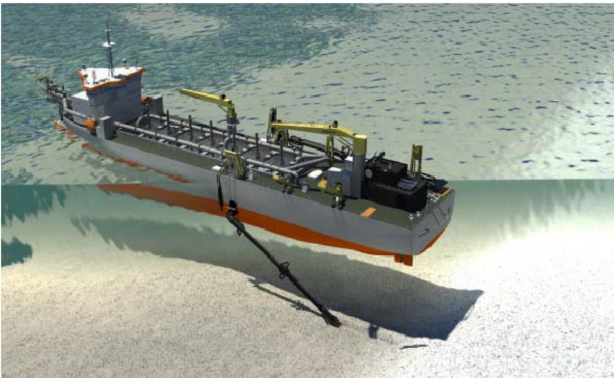
Figure 55 Trailing Suction Hopper Dredger
