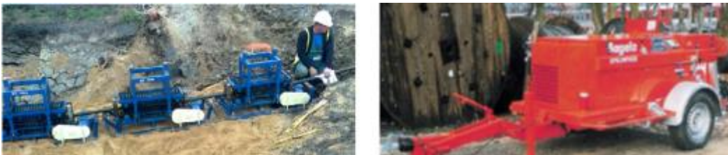
Figure 18 Typical cable tensioners (left) & cable winch (right)
