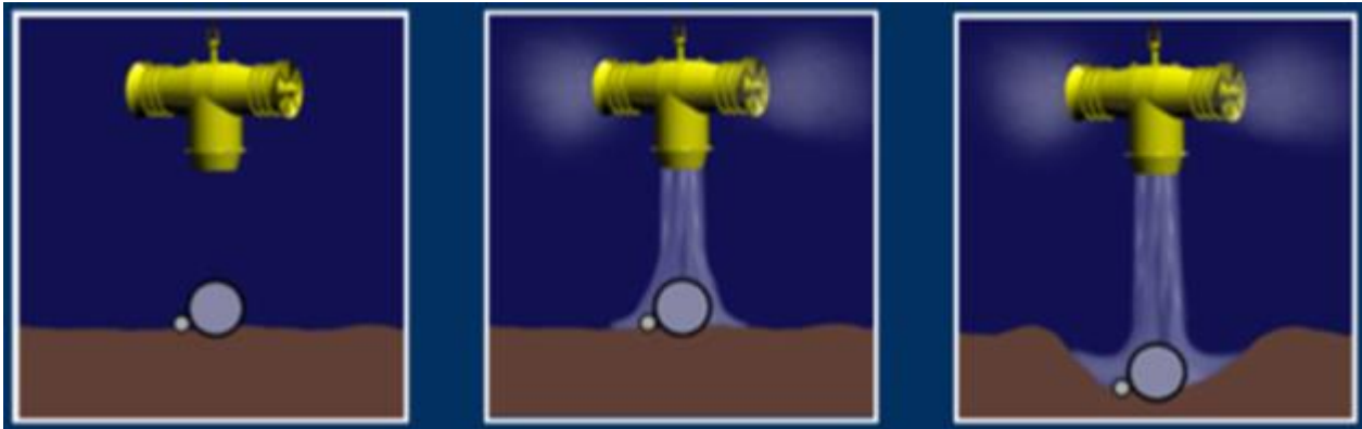
Figure 46 Mass flow excavation
