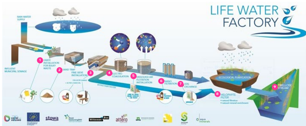
Figure 5 Schematic diagram of unit processes in the sewage water treatment at the Water Factory Wilp. 1-2) Screens and sand trap units; 3) fine sieve installation to remove cellulose; 4) electrocoagulation unit that promotes the coagulation and flocculation of phosphate and organic material; 5) dissolved air flotation (DAF) unit; 6) nanofiltration unit; 7) ion-exchange process for ammonium removal; 8) helophyte filter; 9) clean water is released (Figure taken from [126])
