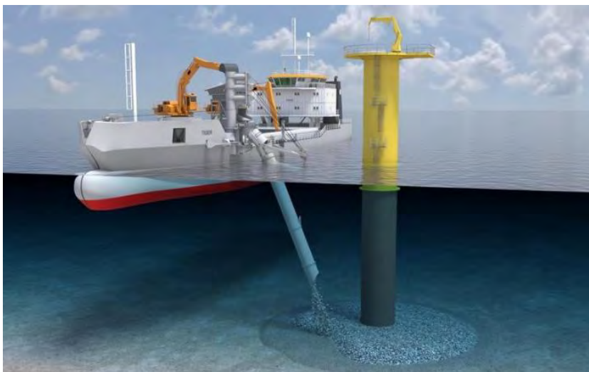
Figure 5 Rock installation vessel with inclined fallpipe
