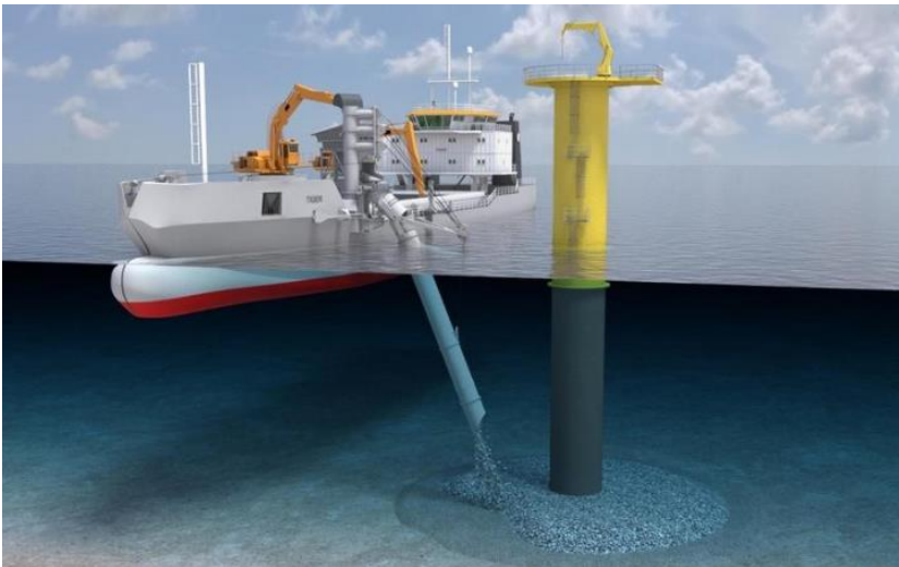
Figure 5 Rock installation vessel with inclined fallpipe
