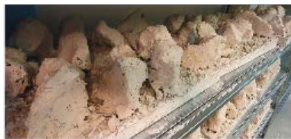
Reefs made from BESE-reef paste ready for the field
