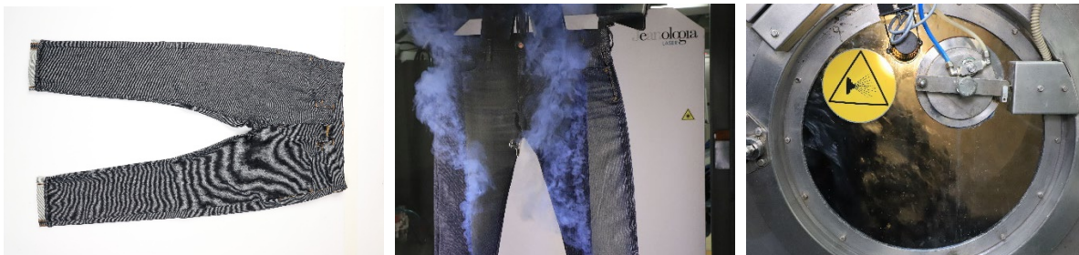
Raw denim jeans; laser treatment; E-Flow washing
