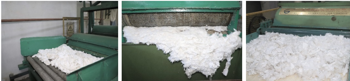
Shredding machine cut down 2-inch pieces of fabric into ½ inch pieces; Output of shredding machine; Fibre opening machine converts ½ inch to fibres.
