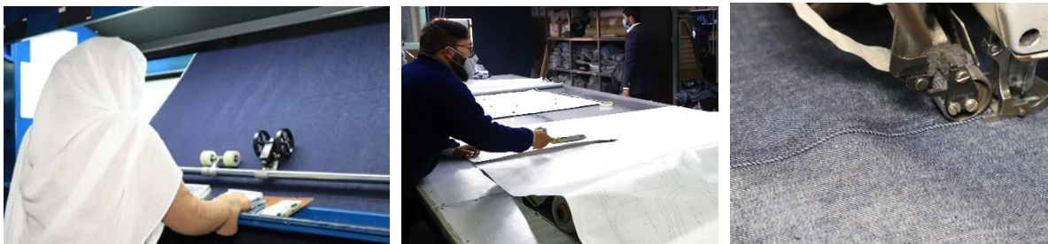
Inspection; cutting; stitching
