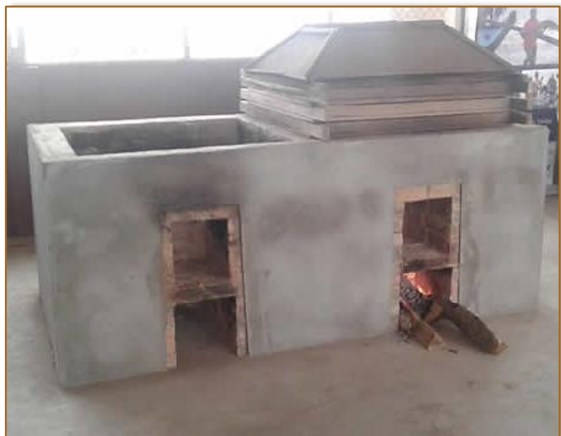
Image 5: Ahotor oven developed by SNV Ghana
