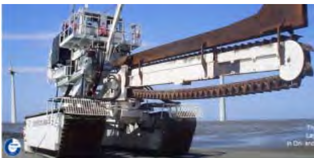
Figure 26 Typical Chain cutter
