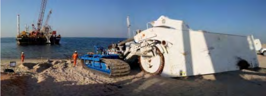
Figure 27 TM04 Wheel cutter cable trencher
