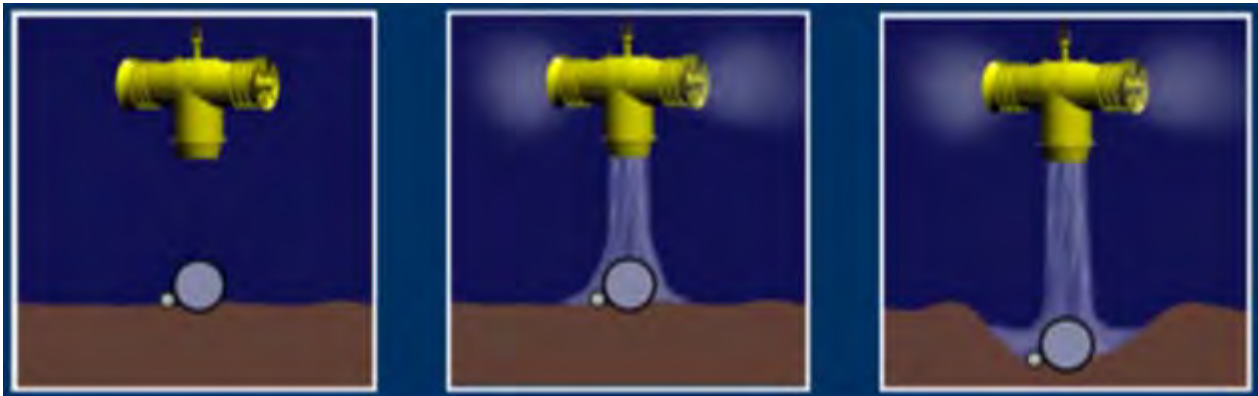
Figure 31 Mass flow excavation
