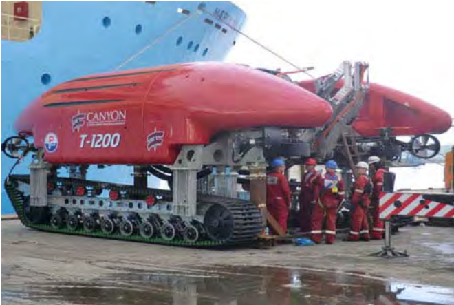
Figure 25 Typical ROV Jet trencher
