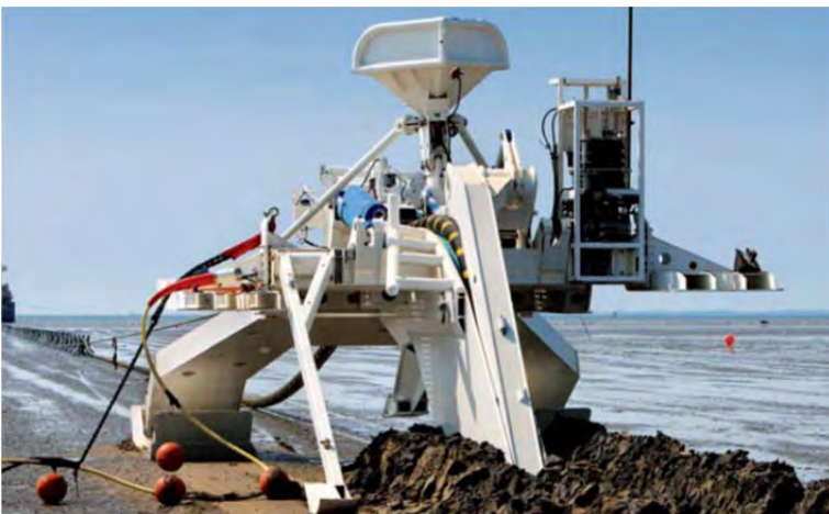
Figure 30 Sea Stallion cable plough
