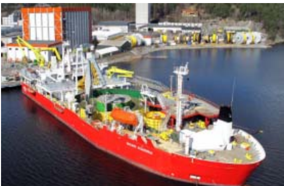
Figure 17 Typical deep water cable installation vessels
