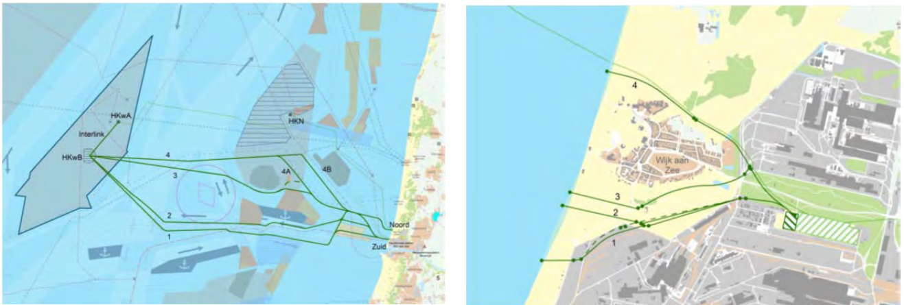
Figure 1 Chart of the different cable route options from the HKwB windfarm to the onshore grid.
