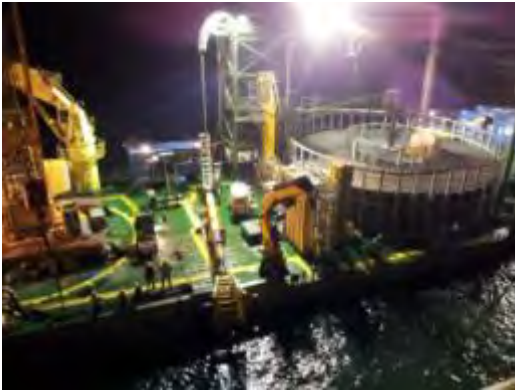
Figure 18 Typical nearshore cable lay barges
