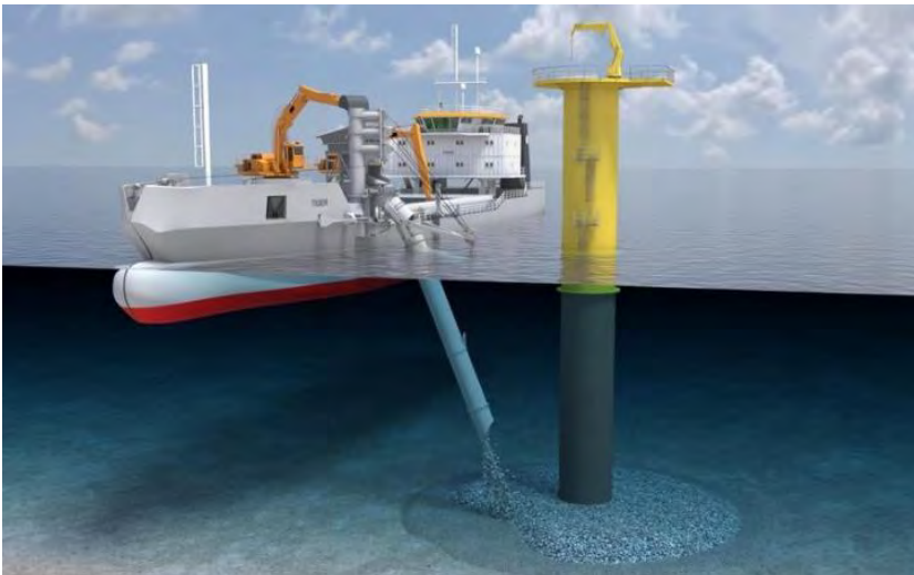
Figure 5 Rock installation vessel with inclined fallpipe
