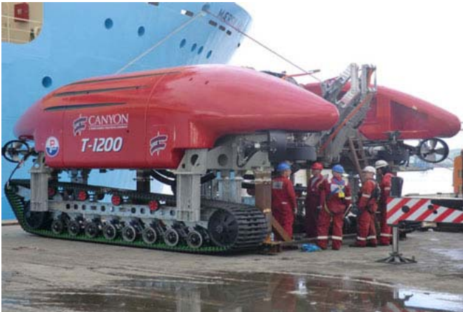
Figure 25 Typical ROV Jet trencher
