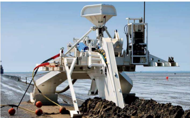
Figure 30 Sea Stallion cable plough
