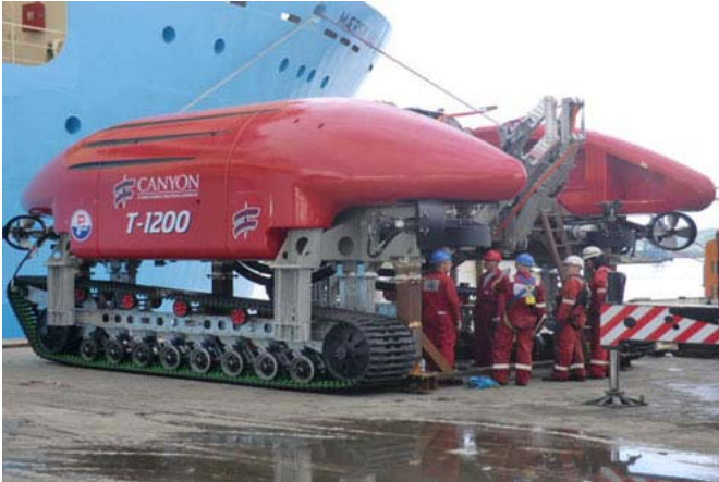
Figure 25 Typical ROV Jet trencher
