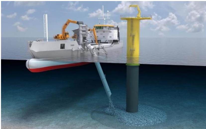
Figure 5 Rock installation vessel with inclined fallpipe
