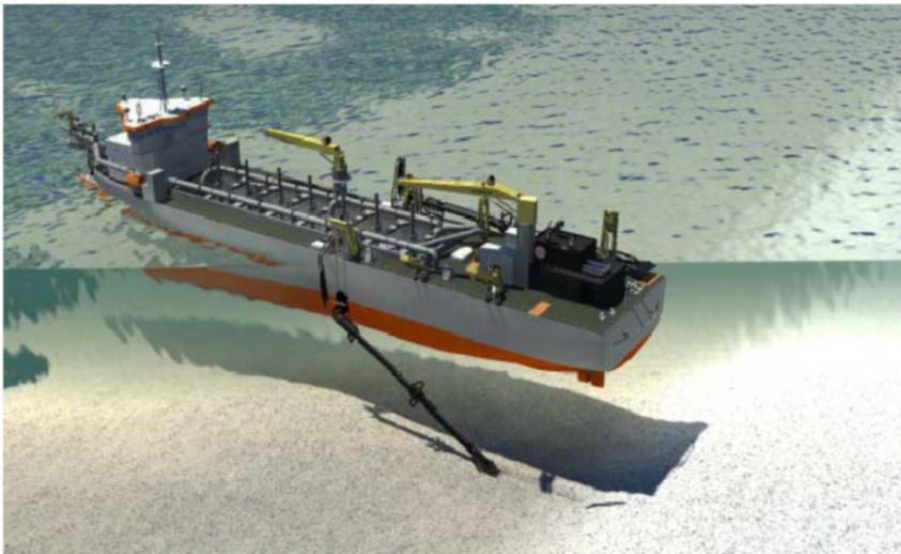
Figure 14 Trailing Suction Hopper Dredger
