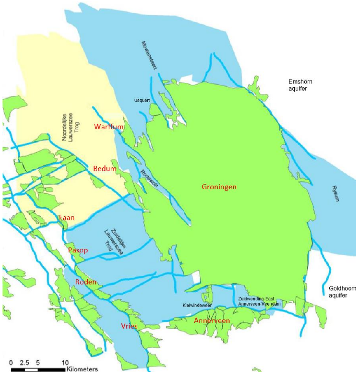
Figure 3-1 Overview of the most important lateral aquifers attached to the Groningen field. In red the field names that are mentioned in the text.
