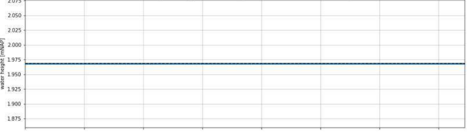
Peak water depth at output location TS9 (water level - bed level a 1.97 mNAP): 0.0 m
