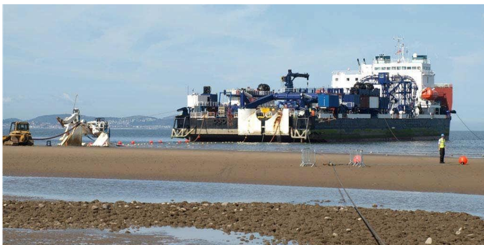
Figuur 5-4 Typische nearshore CLV (Cable Lay Vessel)
