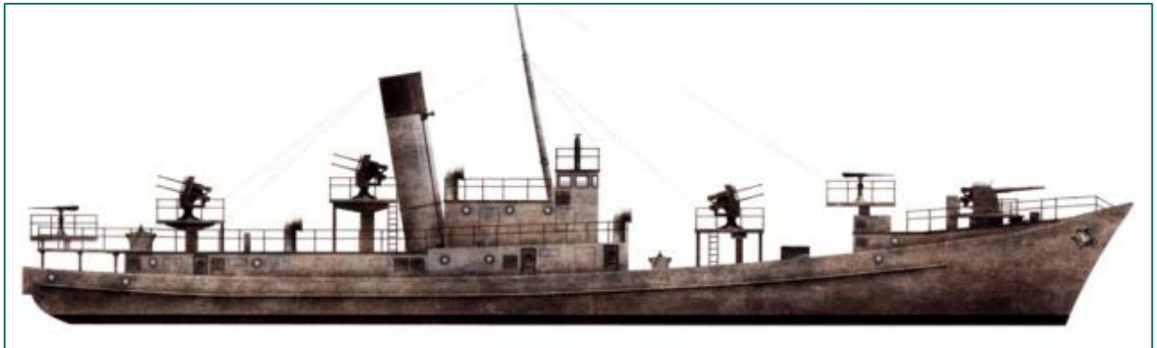
Figure 5: Illustration of a German Vorpostenboot, which was in fact a heavily armed trawler. (Source: http://prussia.online/Data/Book/kr/kriegsmarine-coastal-forces/NV151%20-20Kriegsmarine%20Coastal%20Forces.pdf ).
