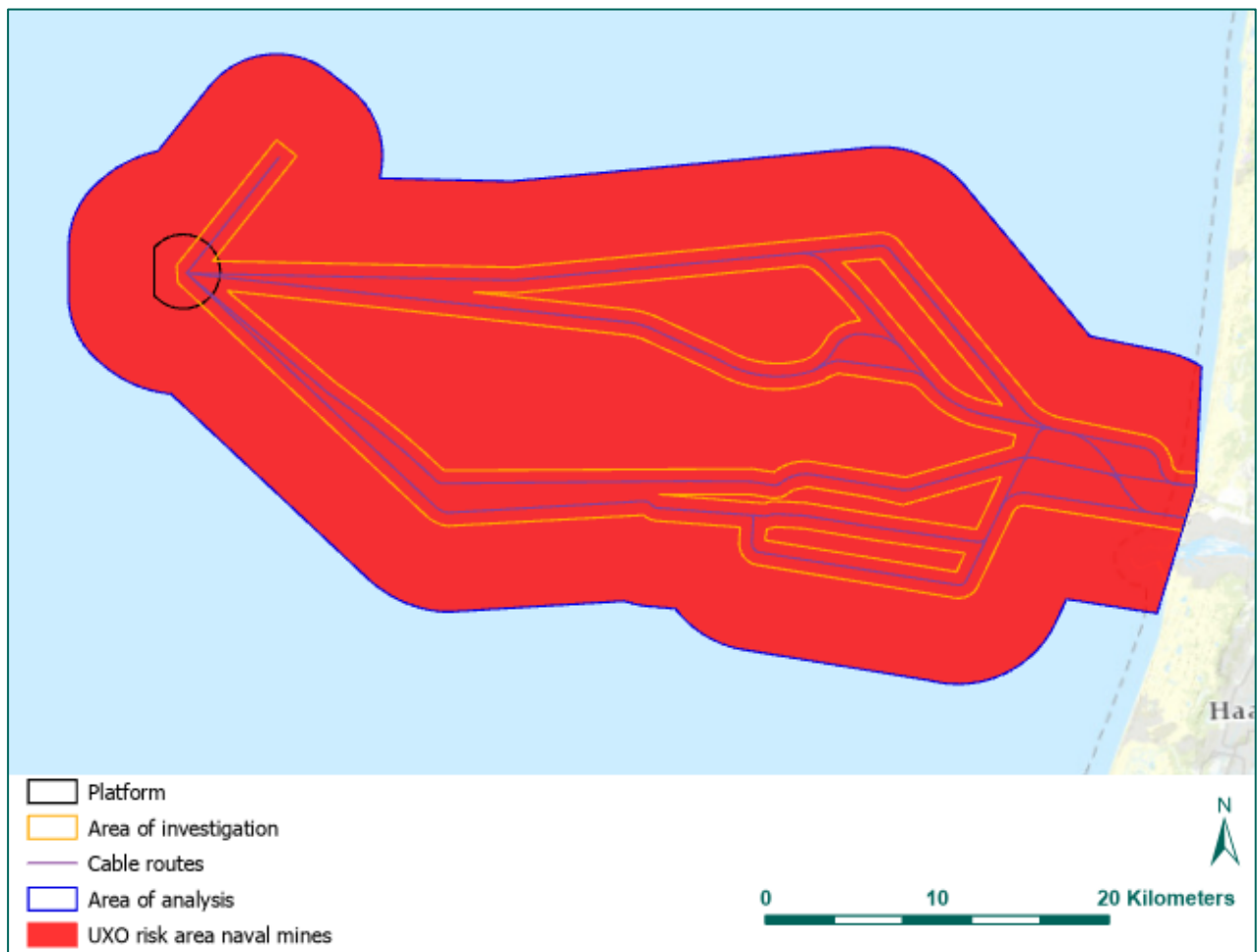
Figure 33: UXO risk area caused by naval mines. (Source basemap: ESRI).
