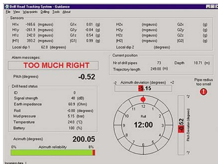
Figure 3. Guidance display of present magnetometer based navigation system. When the azimuth and pitch deviation is kept at zero, the desired track is followed. The reliability bar indicates whether a disturbance of the Earth's magnetic field exists.
