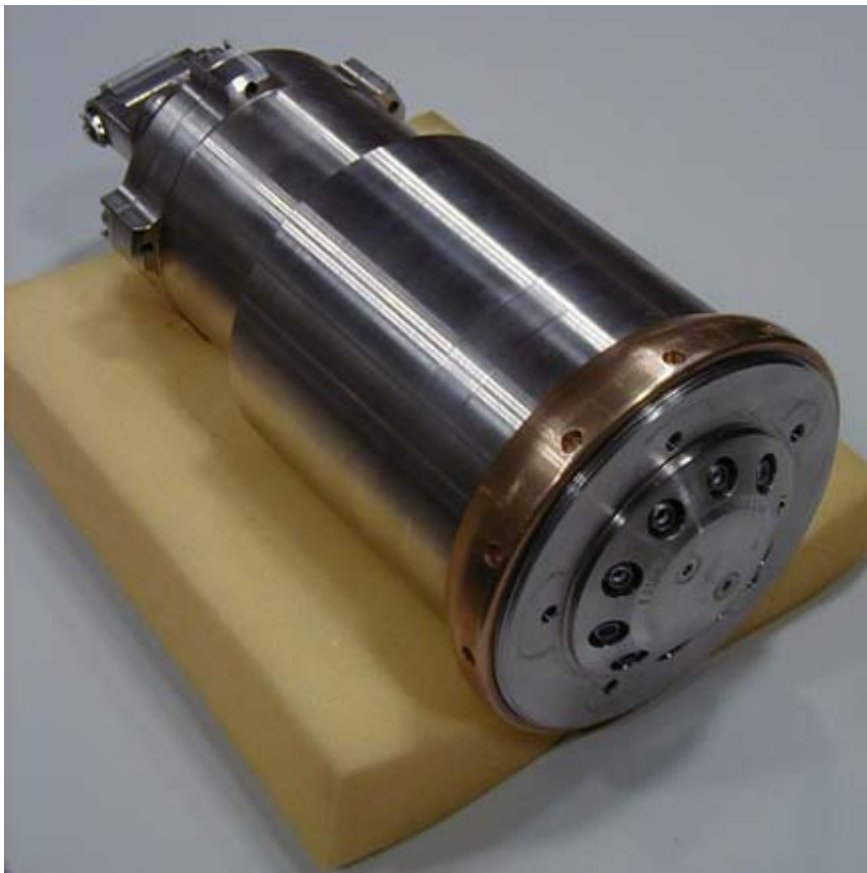
Figure 2. Probe with Ring Laser Gyroscope, the robust housing is suitable for a rough environment with high vibrations and shock loading. The unit contains three perpendicular installed RLG's and three perpendicular installed servo-balanced accelerometers, as well as micro-controllers for processing and filtering of the measured data. The total unit is build into the drillstring close to the drillhead. This drillstring part contains a second micro-controller for processing of strain gage and mud pressure signals, as well as for modulation and transmission.
