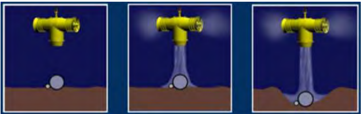
Figure 43 Mass flow excavation
