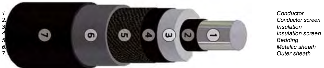
Figure 6 Typical HVAC 220 kV land export cable
