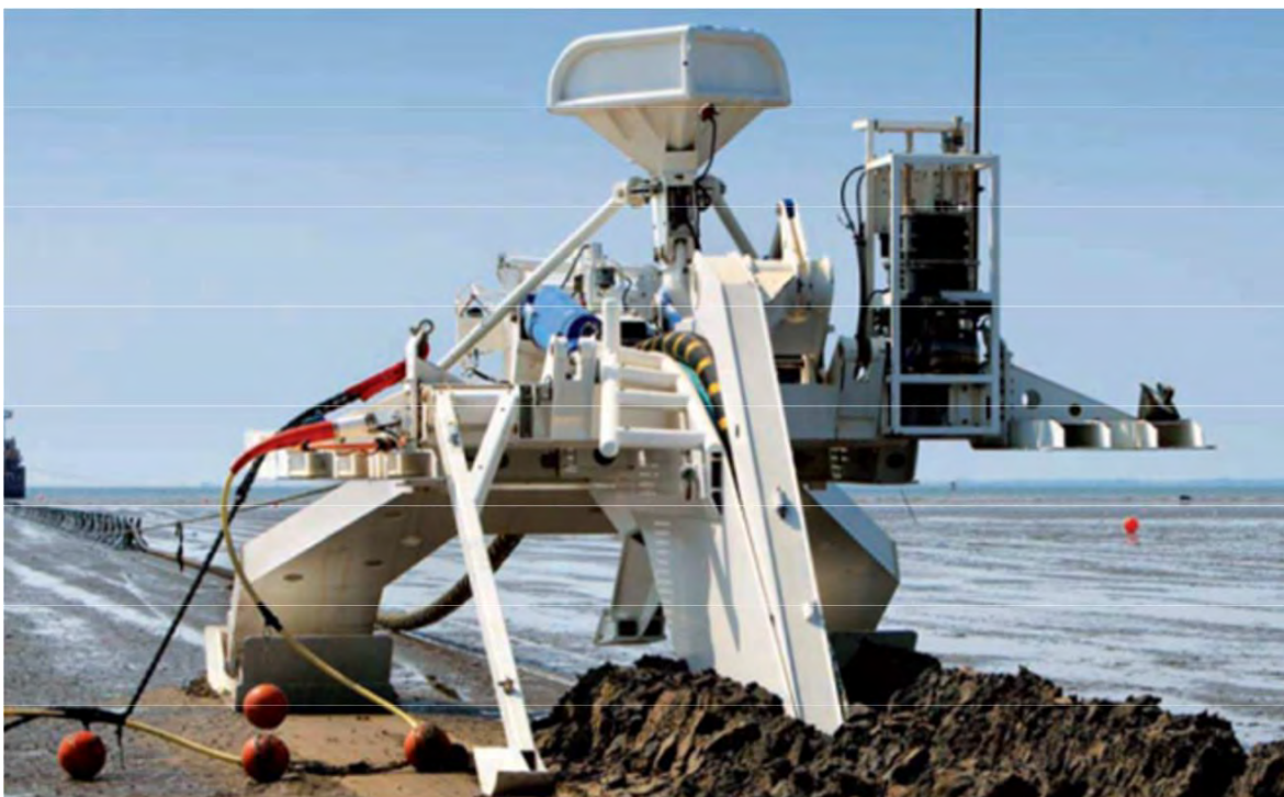
Figure 42 Sea Stallion cable plough
