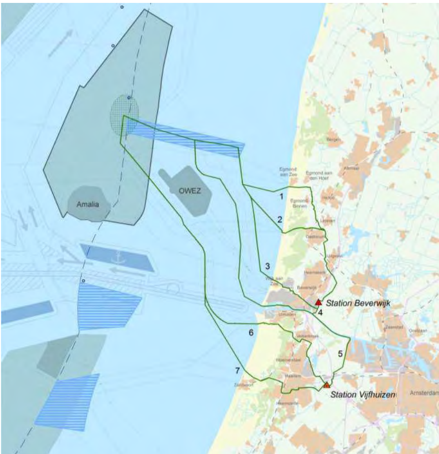
Figure 1 Chart of the different cable route options from the HKN windfarm to the onshore grid
