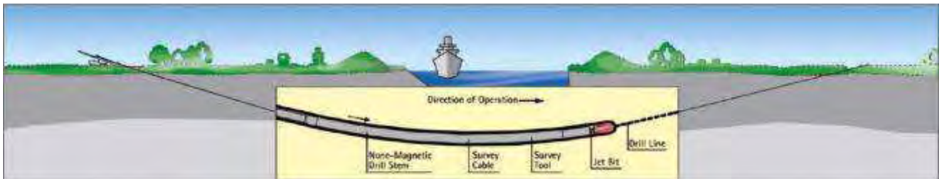
Figure 23 First stage of a HDD - pilot drill
