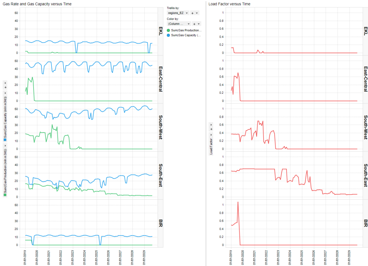
Figure 3-32: Utilisation of the various production regions for Strategy 2 (Event count), warm temperature year.
