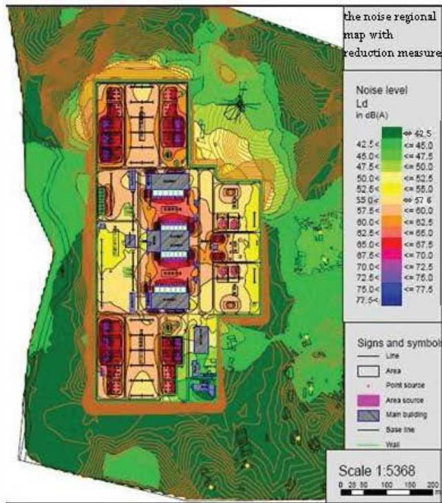
Figure 4 The noise map with taking noise reduction measures
