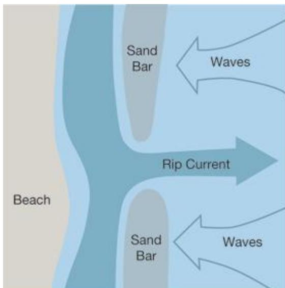
Figure 3.15: Rip currents occur between two sand banks. Locally, the seabed is lower than its surroundings.
