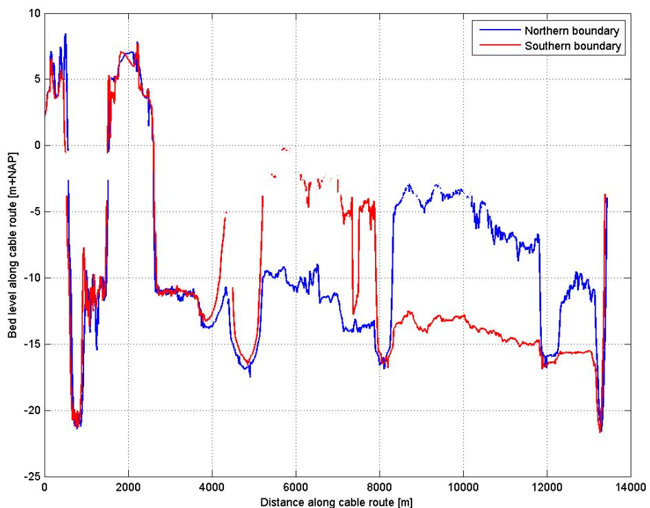
Figure 4.3: Depth (bed level 2017) along cable route alternative 5 in IJmuiden Port and the Noordzeekanaal.
