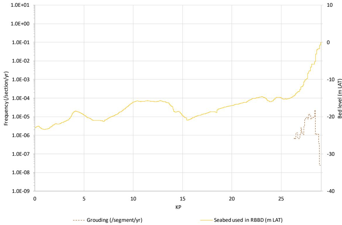
**Figure 5.5** Frequency that critical ship grounding occurs on Hollandse Kust (noord) route alternative 2.
