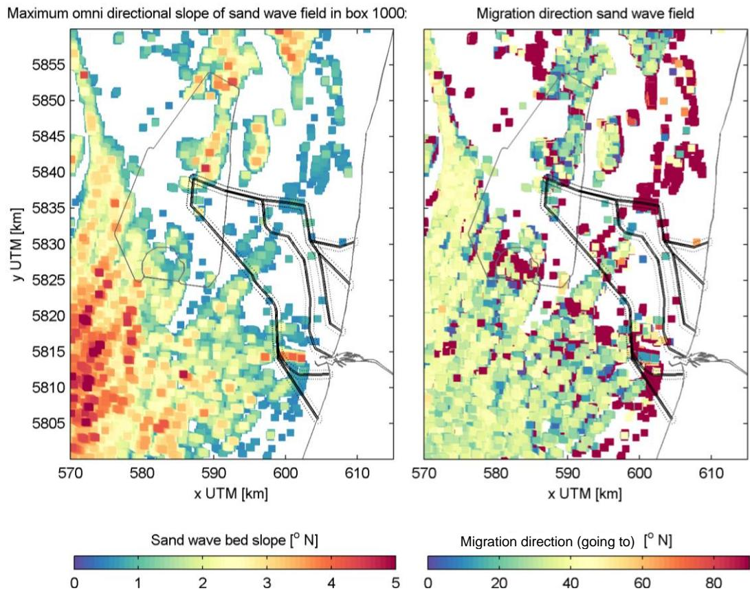
Figure 2.7 Left panel: Steepest bed slope in boxes of 1000x1000m. Right panel: Migration direction sand waves determined from the direction of the steepest bed slope in boxes of 1000x1000m.
