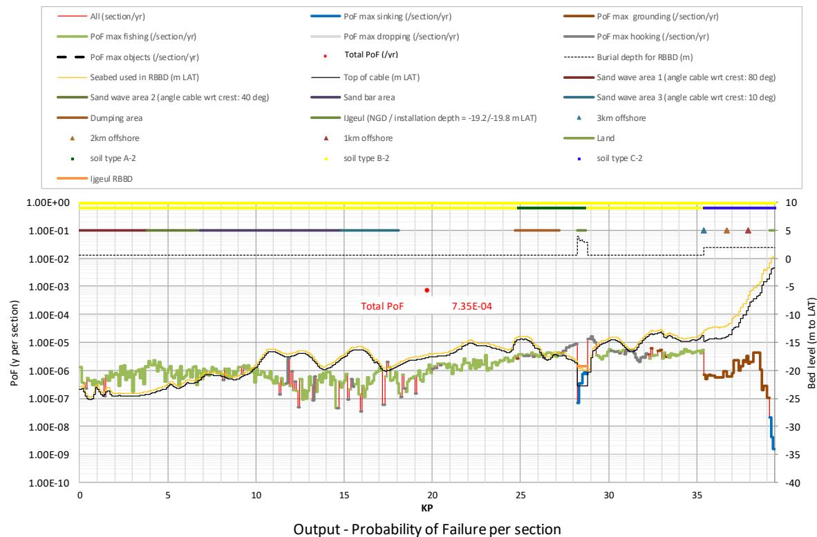
**Figure A2.48****Probability of Failure (PoF) for Hollandse Kust (noord) route alternative 7:**
