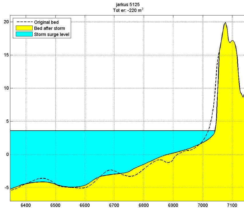
Figure 3.19: Model results of the impact of a 1/100 years storm condition on the most recent recorded coastal profile at landfall location 3.
