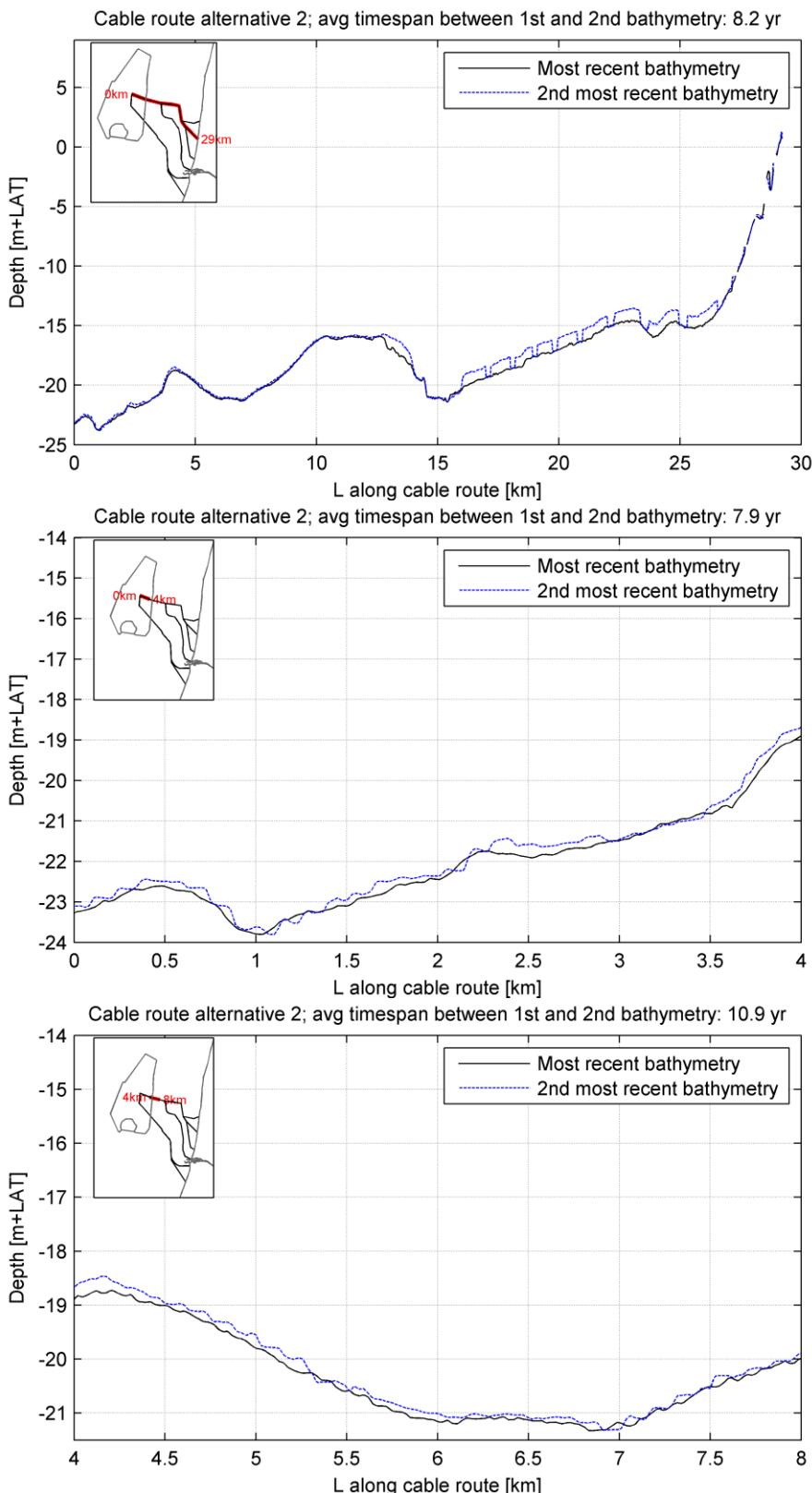
Cable route alternative 2; avg timespan between 1st and 2nd bathymetry: 11.1 yr
