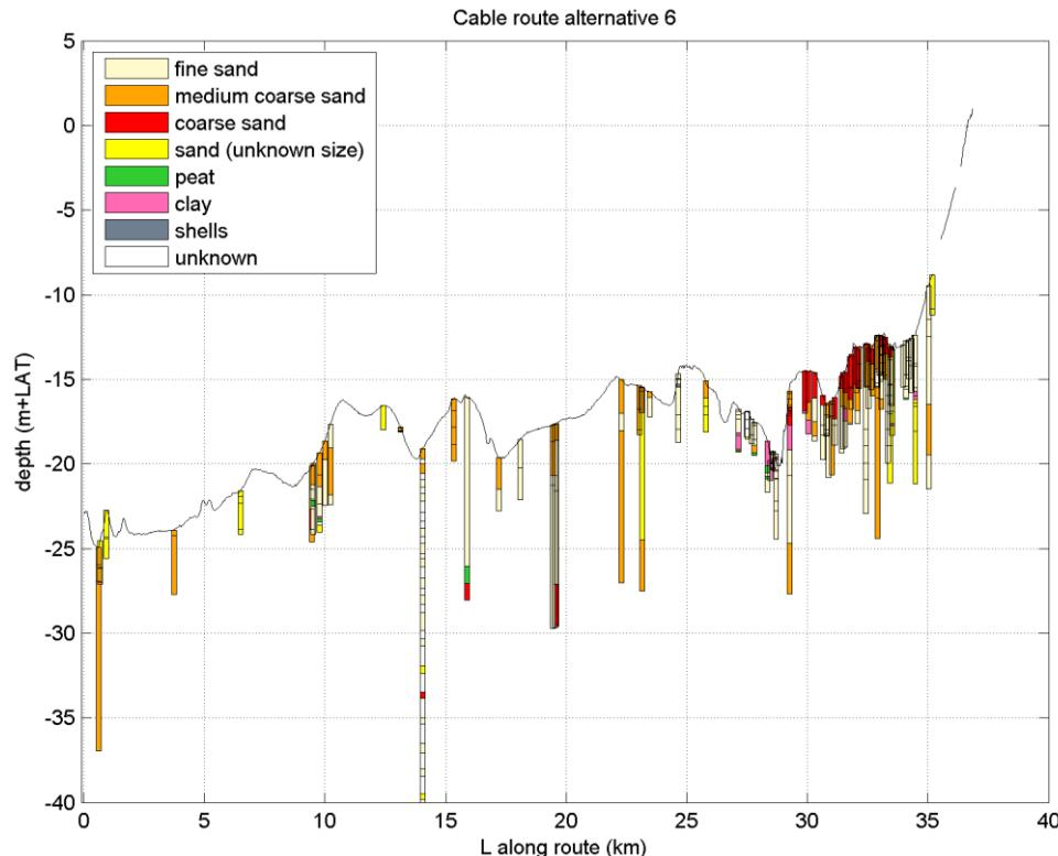
Figure 5.8: Bathymetric and borehole cross-section from O-E, showing mainly medium sand at the surface offshore and coarser sands closer to the coast. IJmuiden shipping channel is visible around km 29, with deposits of clay belonging to the Layer of Velsen (part of the Naaldwijk formation) which have become exposed due to dredging activities. Below the clay, remnants of peat from the Nieuwkoop formation can be seen.
