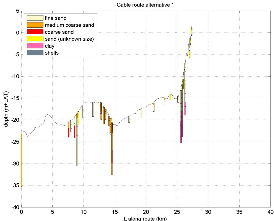
Figure 5.4: Bathymetric and borehole cross-section from O-A, showing mainly fine and medium sand at the surface and some coarser sand at 2 m depth. Near shore clay formation of the Layer of Velsen (part of the Naaldwijk formation) is apparent at 8m depth.
