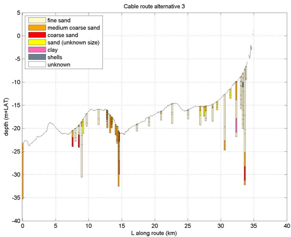
*Figure 5.6: Bathymetric and borehole cross-section from O-C, showing mainly medium sand at the surface. Near shore some small patches of clay of the Layer of Velsen (part of the Naaldwijk formation) is apparent at 8 m depth.*
