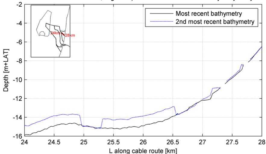
Cable route alternative 2; avg timespan between 1st and 2nd bathymetry: 0.7 yr
