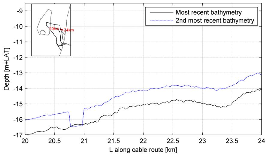
Cable route alternative 1; avg timespan between 1st and 2nd bathymetry: 4.4 yr
