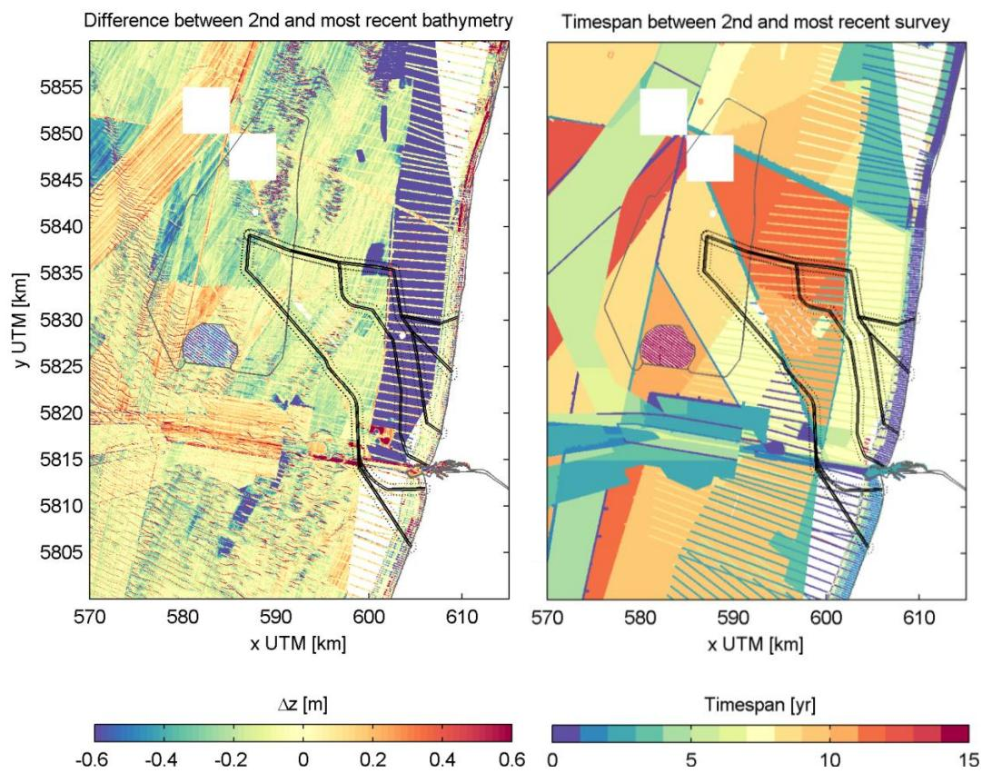
Figure 2.4 Left panel: Difference between most recent and 2<sup>nd</sup> most recent bathymetry map showing change in bed level over time. Right panel: Time span between most recent and 2<sup>nd</sup> most recent bathymetry.
