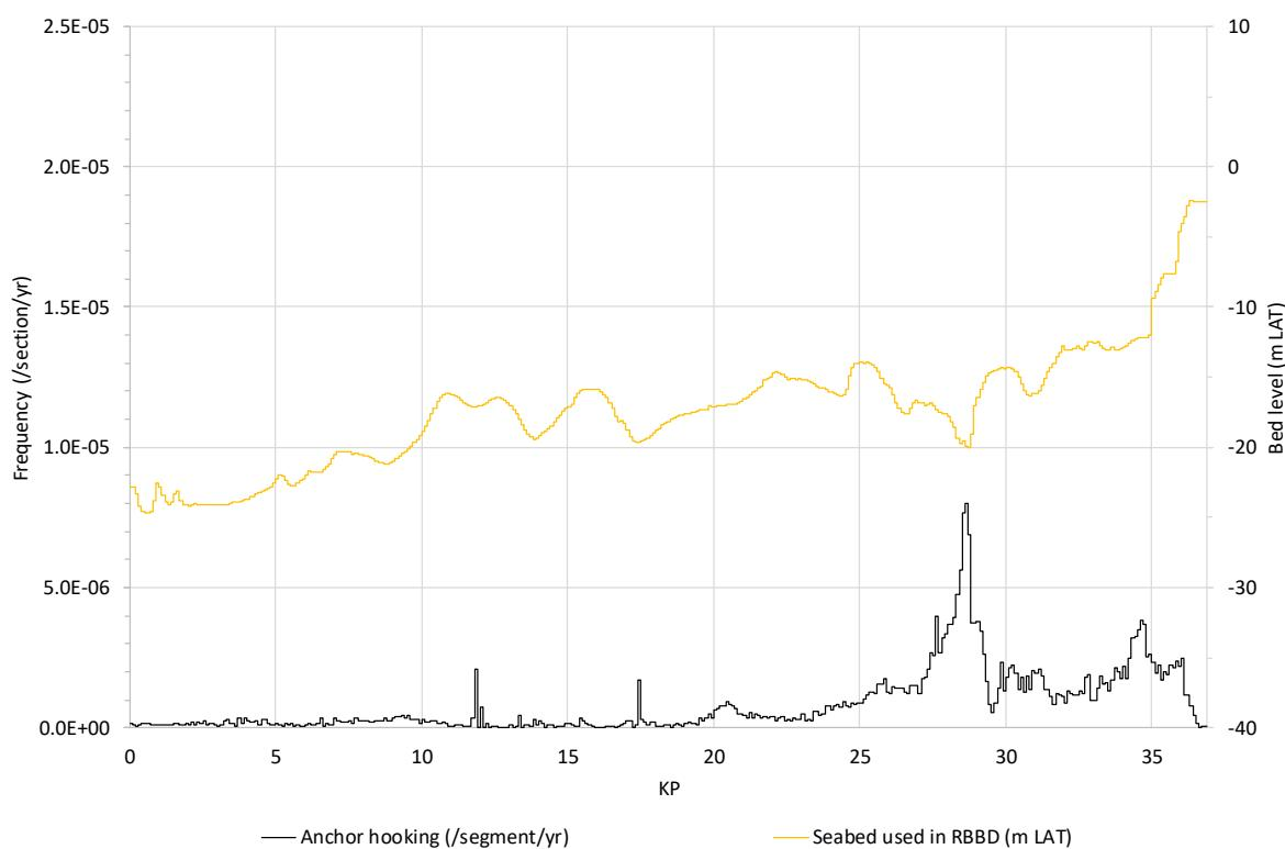
**Figure 5.13** Frequency that critical anchor hooking occurs on Hollandse Kust (noord) route alternative 6.
