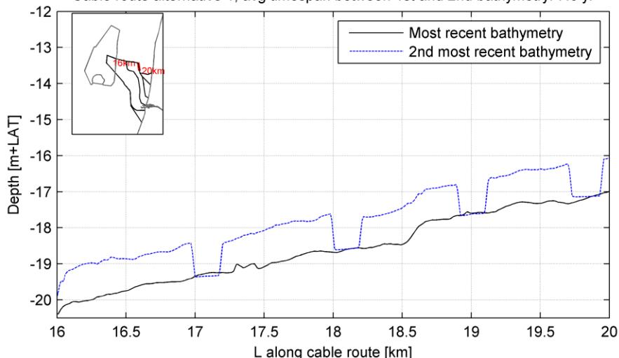
Cable route alternative 1; avg timespan between 1st and 2nd bathymetry: 7.9 yr
