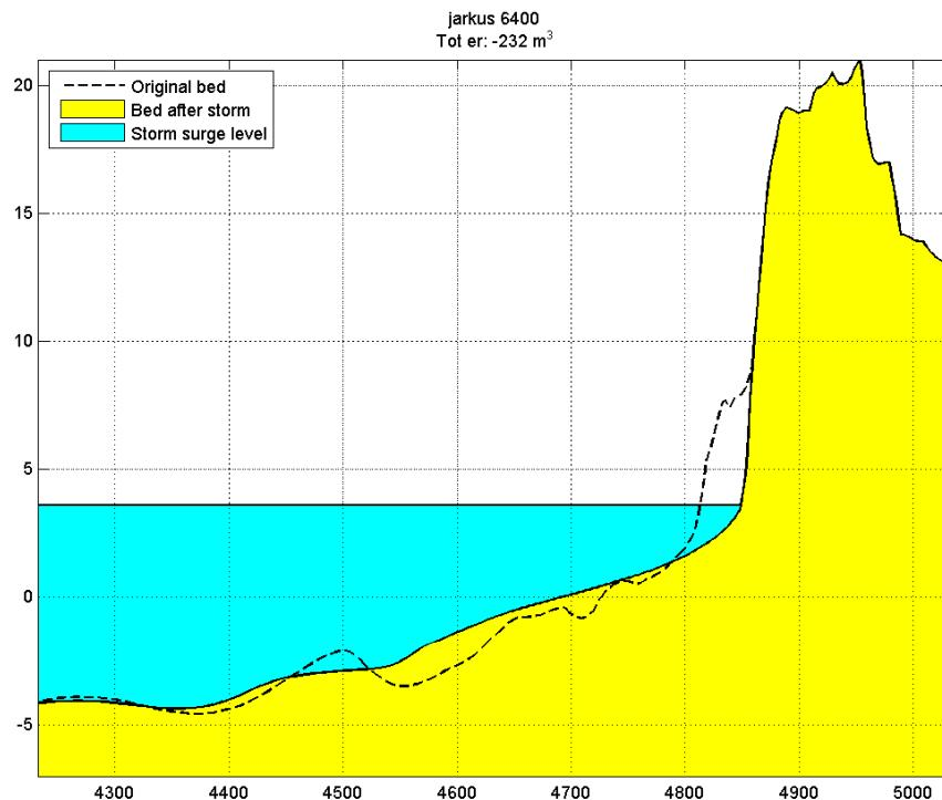
*Figure 3.22: Model results of the impact of a 1/100 years storm condition on the most recent recorded coastal profile at landfall location 7.*
