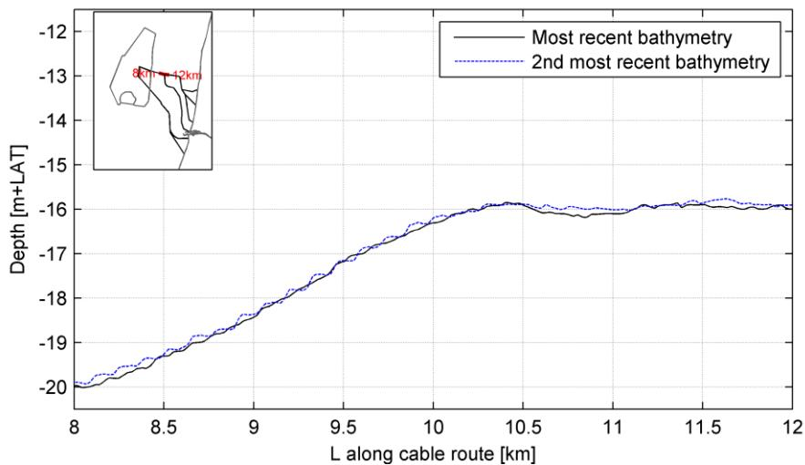
Cable route alternative 3; avg timespan between 1st and 2nd bathymetry: 7.4 yr
