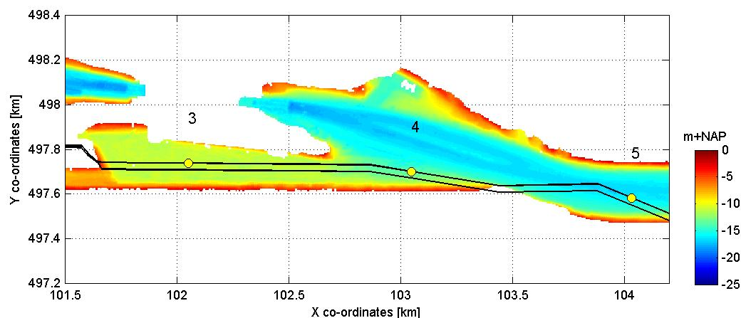
Figure 4.9: Bed level (2017) of IJmuiden locks and Noordzeekanaal with the cable route alternative 4 and 5 (black) and KP's.
