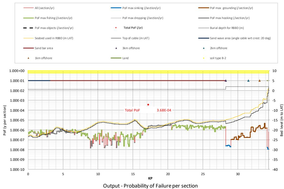
**Figure A2.45****Probability of Failure (PoF) for Hollandse Kust (noord) route alternative 3:**
