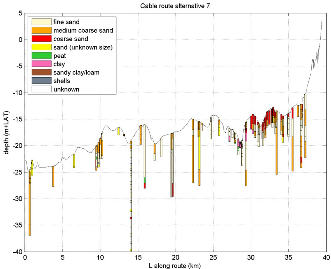
*Figure 5.9: Bathymetric and borehole cross-section from O-F, showing mainly medium sand at the surface offshore and coarser sands closer to the coast. IJmuiden shipping channel is visible around km 29, with deposits of clay belonging to the Layer of Velsen (part of the Naaldwijk formation) which have become exposed due to dredging activities. Below the clay, remnants of peat from the Nieuwkoop formation can be seen.*
