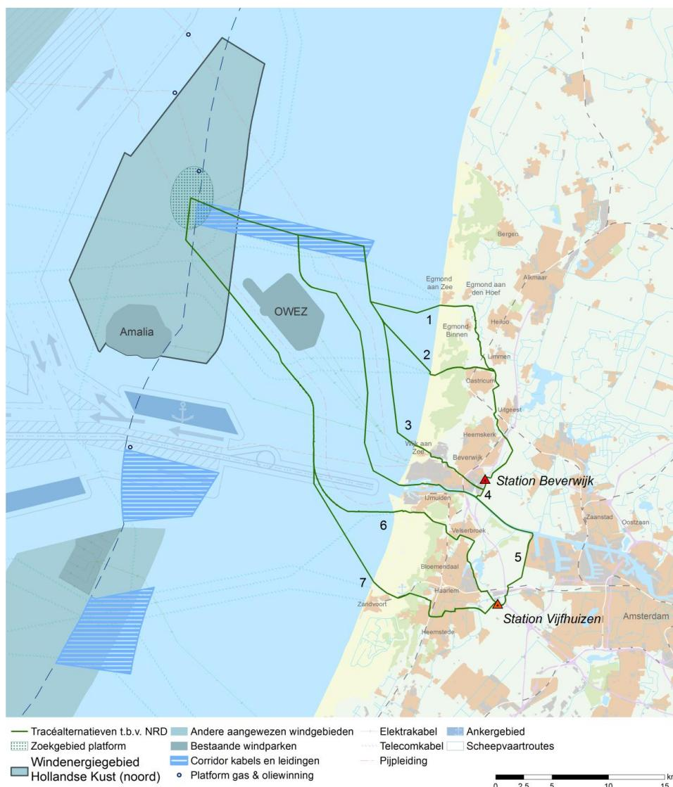
Figure 1.1 Different cable route options windfarm HKN under consideration by TenneT. Source: TenneT TSO B.V.
