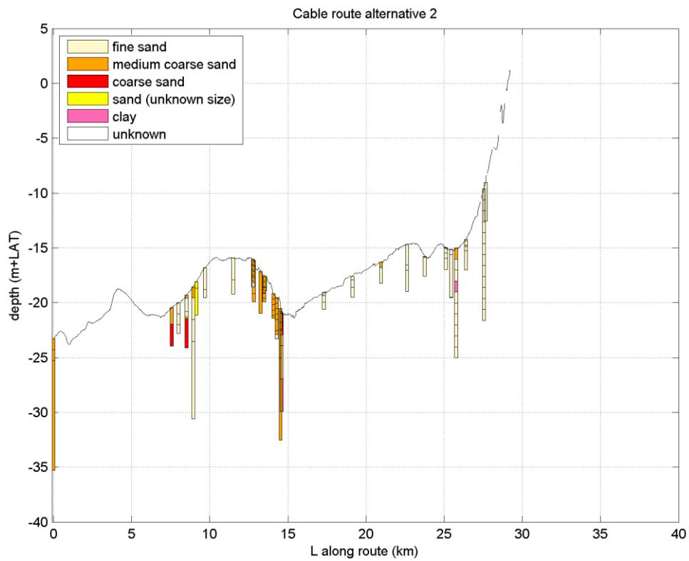
*Figure 5.5: Bathymetric and borehole cross-section from O-B, showing mainly medium sand at the surface and some coarser sand at 2 m depth. Near shore some small patches of clay of the Layer of Velsen (part of the Naaldwijk formation) is apparent at 4 m depth.*
