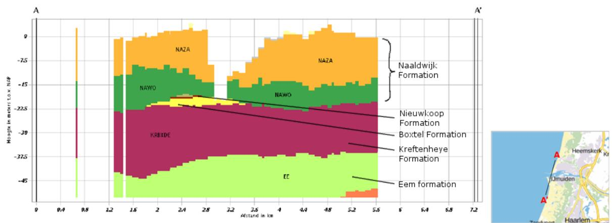
Figure 5.2: Extend of formation along a crosssection over the IJmuiden port Area based of GeoTOP v1.3 accessed via DINO loket<sup>3</sup>.
