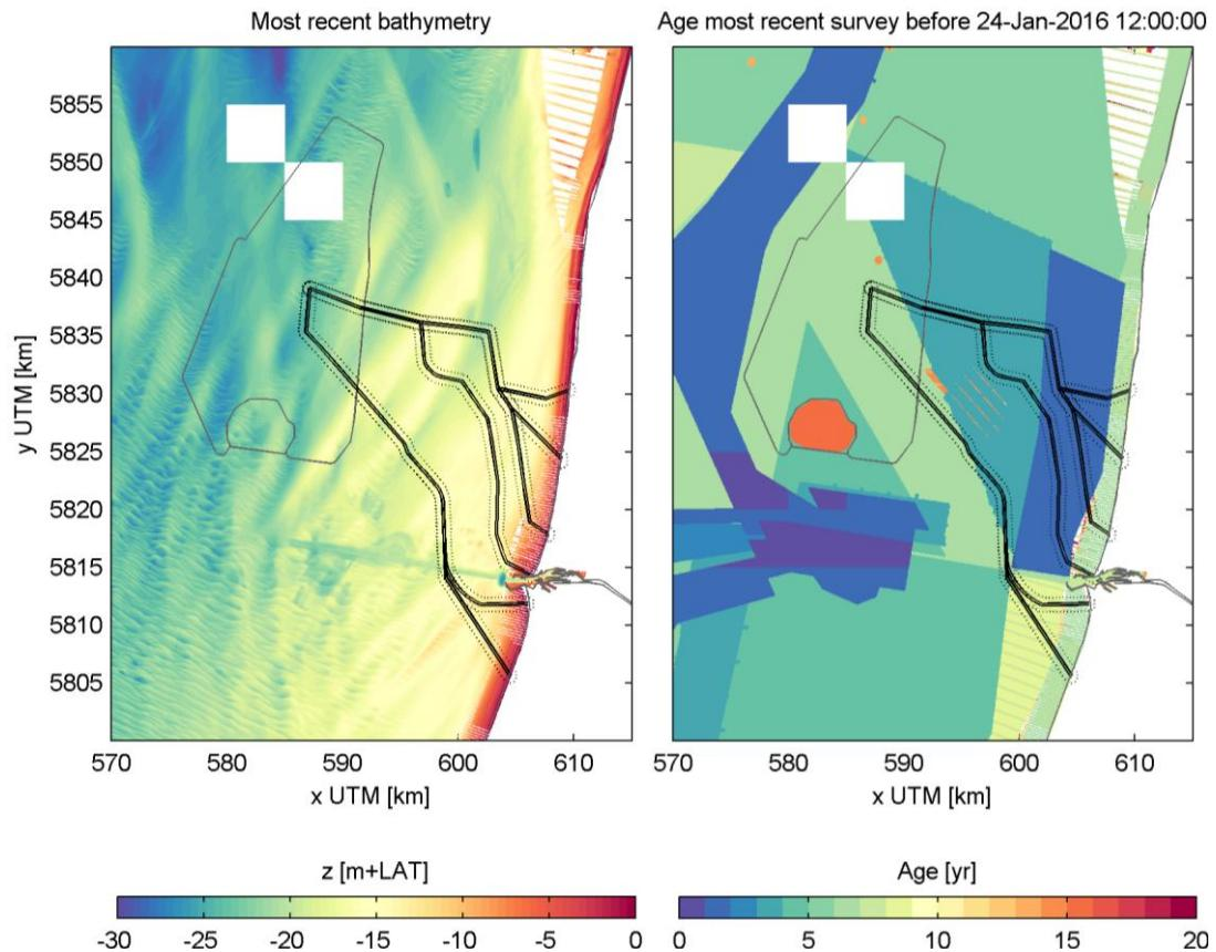
Figure 2.1 Left panel: Most recent bathymetry map. Right panel: Age of composite bathymetry data.
