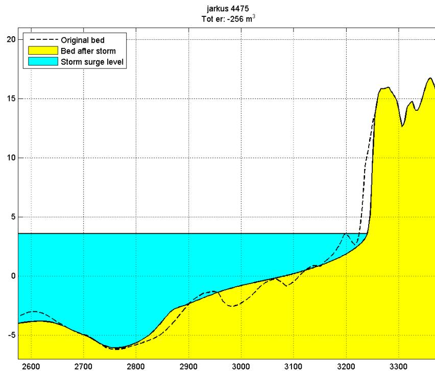
Figure 3.18: Model results of the impact of a 1/100 years storm condition on the most recent recorded coastal profile at landfall location 2.
