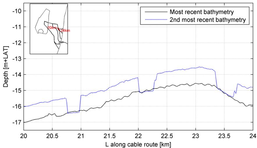
Cable route alternative 2; avg timespan between 1st and 2nd bathymetry: 6.8 yr
