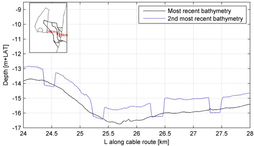
Cable route alternative 5; avg timespan between 1st and 2nd bathymetry: 7.6 yr
