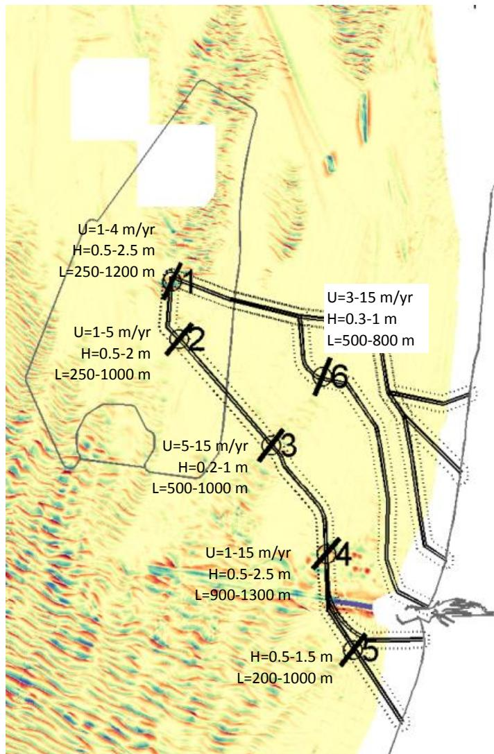
Figure 2.11 Range of sand wave characteristics
