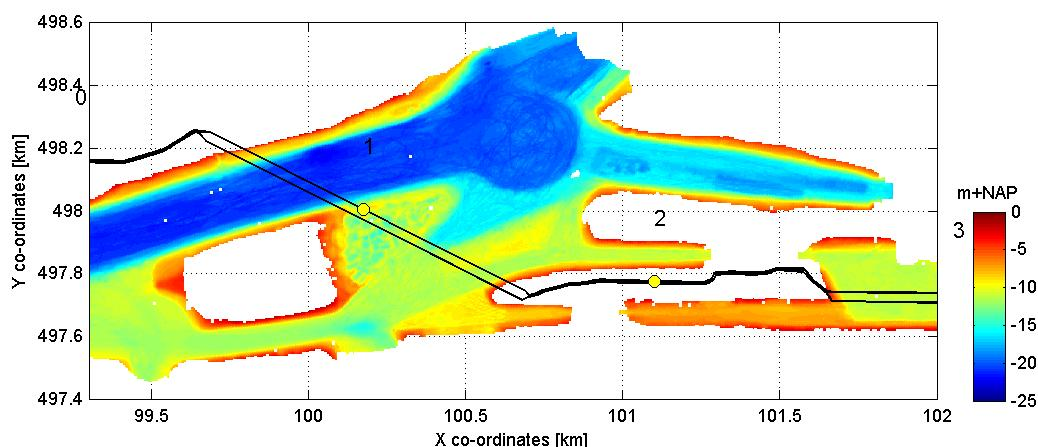
Figure 4.4: Bed level (2017) of IJmuiden Port with the cable route alternative 4 and 5 (black) and KP's.
