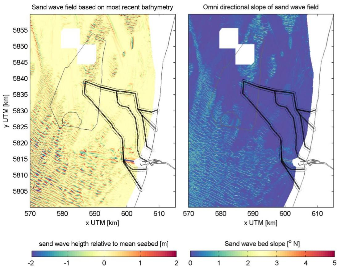
Figure 2.6 Left panel: Sand wave field. Right panel: Bed slopes of sand wave field.
