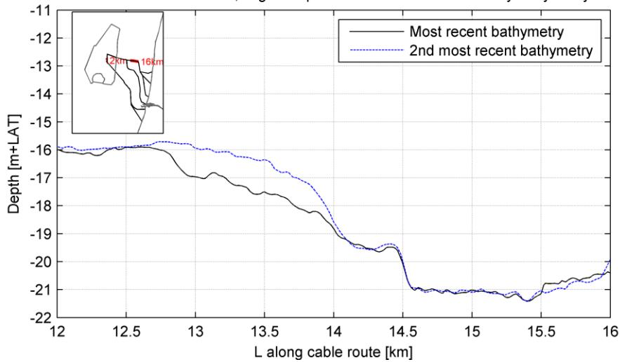
Cable route alternative 2; avg timespan between 1st and 2nd bathymetry: 7.6 yr
