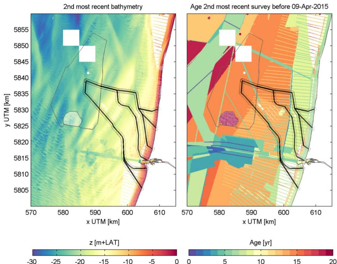
Figure 2.3 Left panel: Second most recent bathymetry map. Right panel: Age of composite bathymetry data
