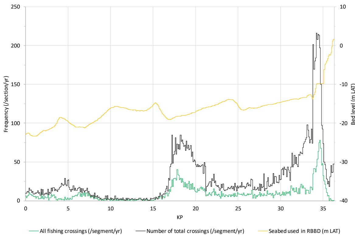
**Figure 5.2** Frequency of all the ships (black line) and fishing ships (green line) that cross route alternative 4 and 5 (/section/yr) as function of the cable route (KP). The numbers are based on two years of AIS data (from 1 January 2015 to 31 December 2016) for each segment of ~100 m. The seabed level (yellow line) that is used for the RBBB is presented in order to link the AIS data to the water depth.
