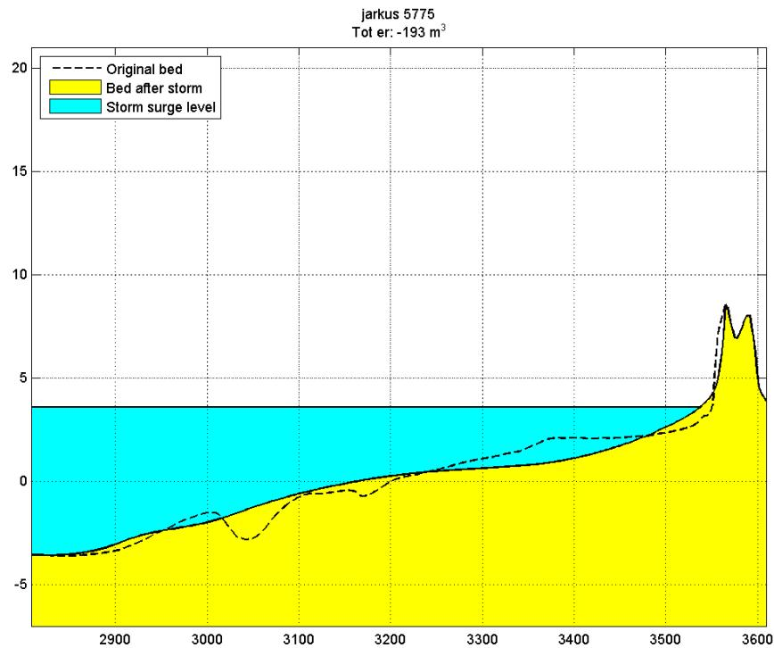
*Figure 3.21: Model results of the impact of a 1/100 years storm condition on the most recent recorded coastal profile at landfall location 6.*
