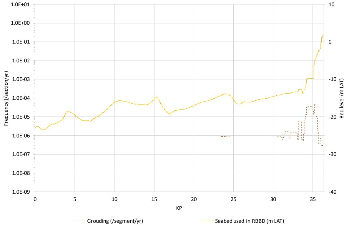
**Figure 5.6** Frequency that critical ship grounding occurs on Hollandse Kust (noord) route alternative 4.
