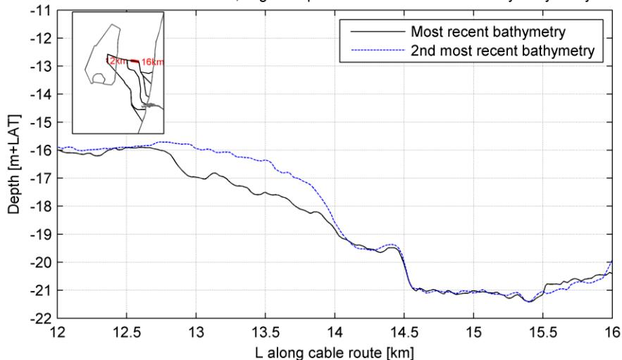
Cable route alternative 1; avg timespan between 1st and 2nd bathymetry: 7.6 yr
