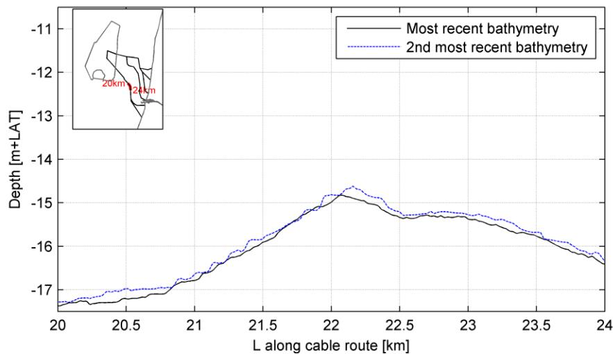
Cable route alternative 7; avg timespan between 1st and 2nd bathymetry: 4.9 yr
