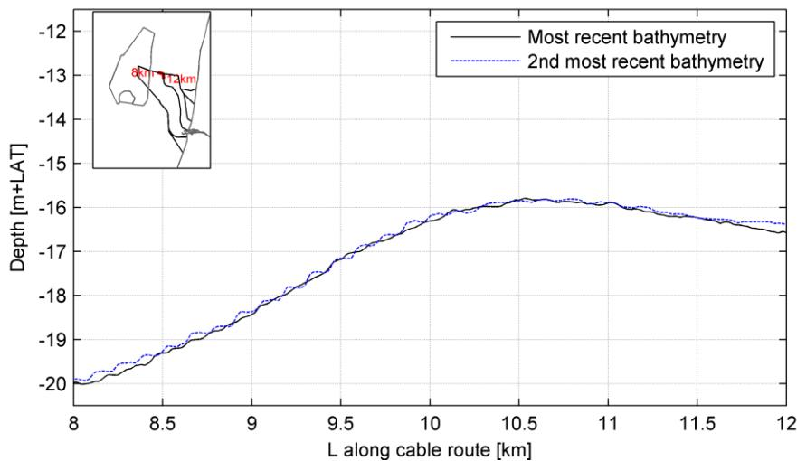
Cable route alternative 4; avg timespan between 1st and 2nd bathymetry: 10.8 yr
