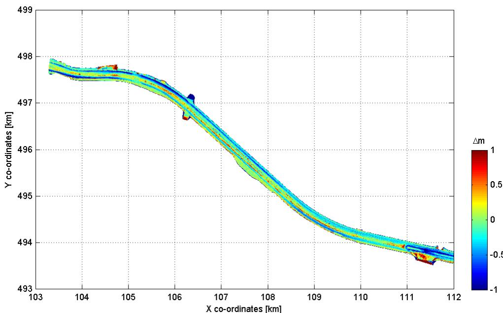
Figure 4.8: Bed level difference in Noordzeekanaal between 2009 and 2017.
