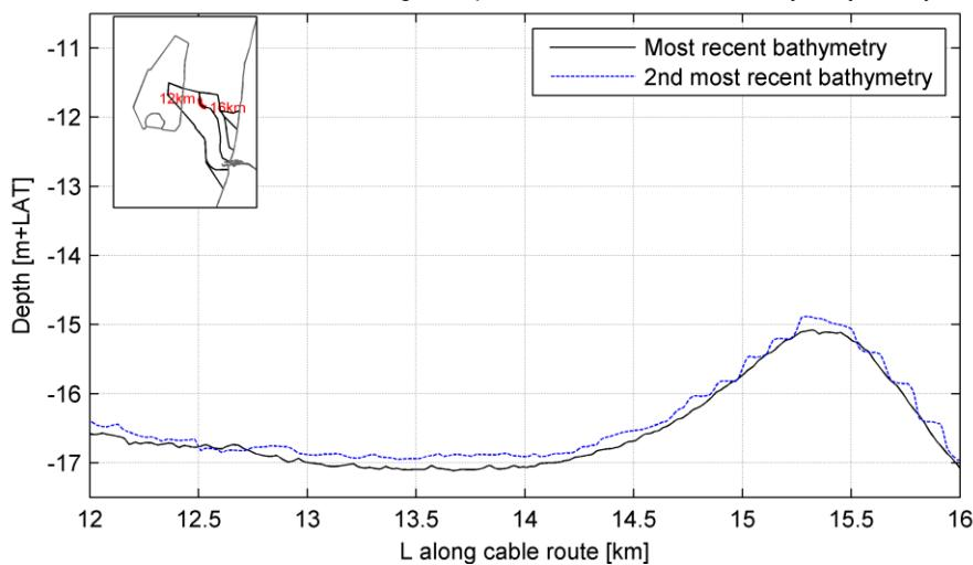
Cable route alternative 4; avg timespan between 1st and 2nd bathymetry: 9.6 yr
