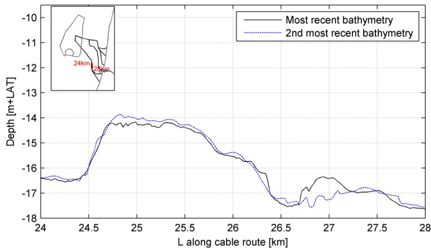
Cable route alternative 7; avg timespan between 1st and 2nd bathymetry: 2.6 yr
