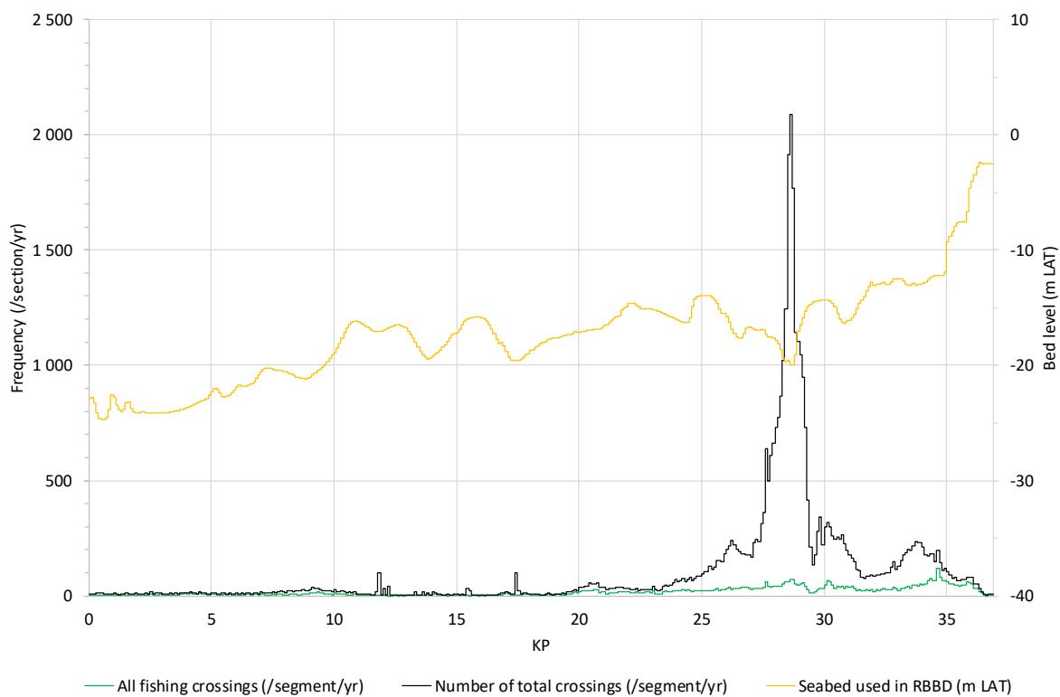
**Figure 5.3** Frequency of all the ships (black line) and fishing ships (green line) that cross
