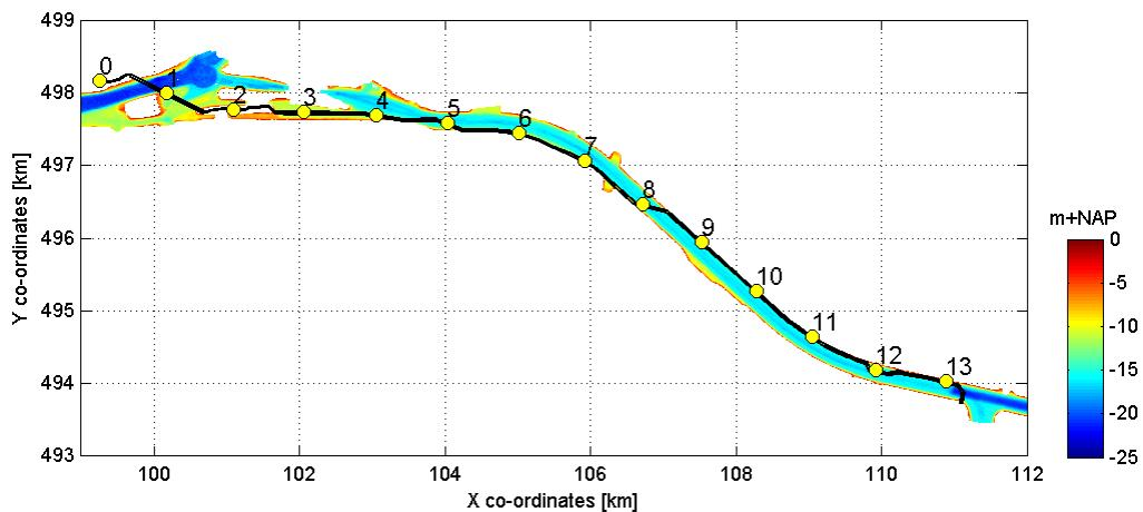
Figure 4.2: Bed level (2017) of IJmuiden Port and the Noordzeekanaal with the cable route alternative 5 (black) and KP's. Alternative 4 follows the same route up to approximately the Wijkertunnel before heading north and reaching land.
