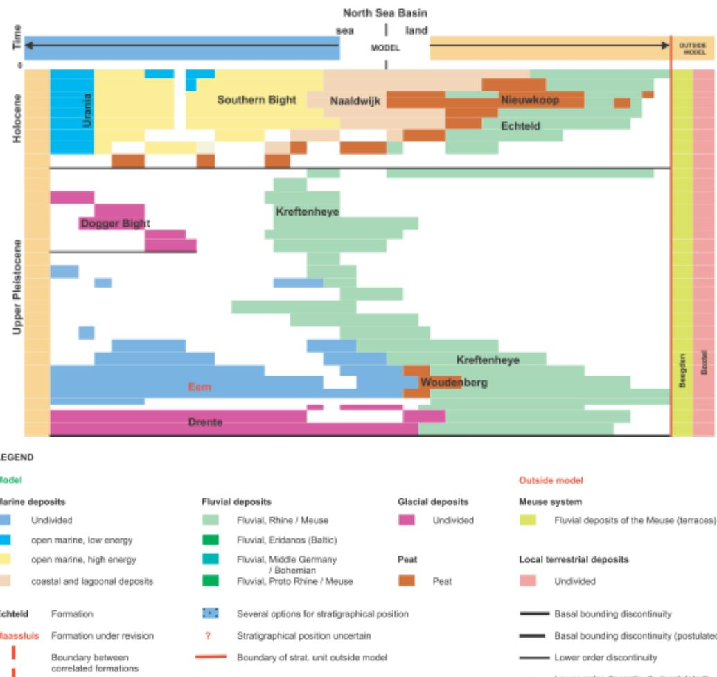
Figure 5.1: Upper part of an integrated stratigraphic model of the North Sea Basin, adapted from Rijssdijk et al. (2005)
