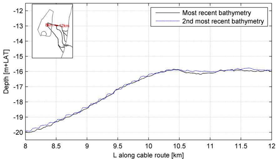
Cable route alternative 1; avg timespan between 1st and 2nd bathymetry: 7.4 yr
