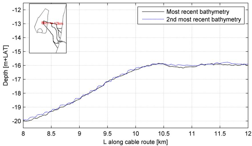
Cable route alternative 2; avg timespan between 1st and 2nd bathymetry: 7.4 yr
