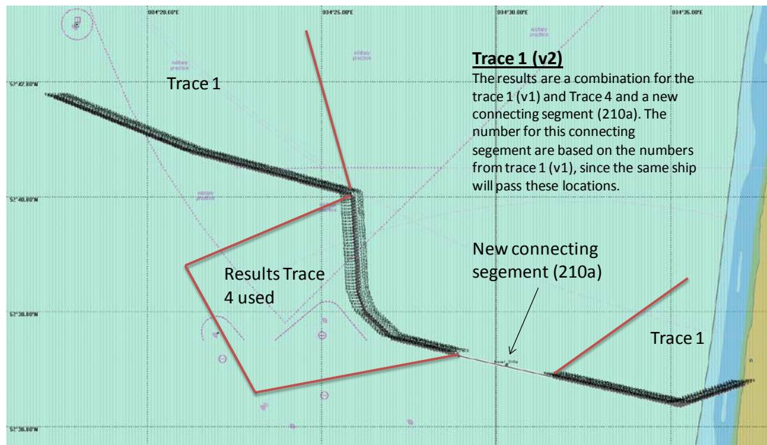
Figuur 4-11 Adjusted segments trace 1
