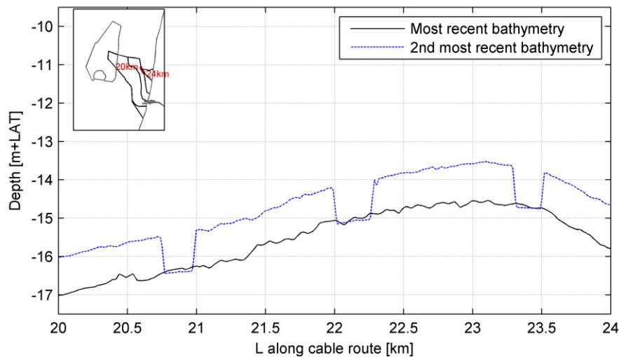
Cable route alternative 3; avg timespan between 1st and 2nd bathymetry: 7.6 yr
