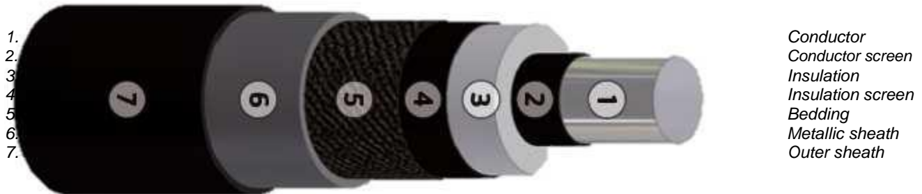
Figure 6 Typical HVAC 220 kV land export cable
