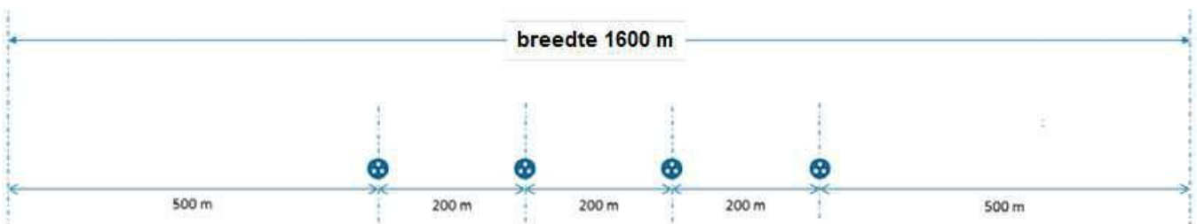
Figure 33 Cable corridor offshore section - 4 cable systems
