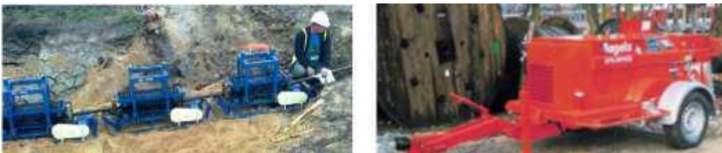
Figure 17 Typical cable tensioners (left) & cable winch (right)
