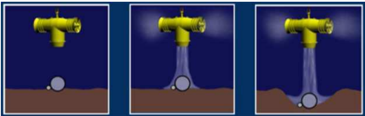
Figure 43 Mass flow excavation
