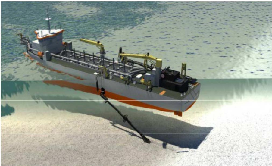
Figure 52 Trailing Suction Hopper Dredger
