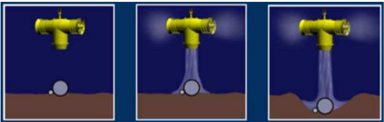
Figure 43 Mass flow excavation
