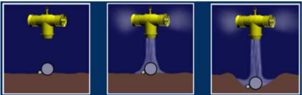
Figure 43 Mass flow excavation
