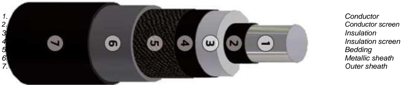
Figure 6 Typical HVAC 220 kV land export cable
