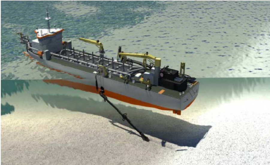
Figure 52 Trailing Suction Hopper Dredger
