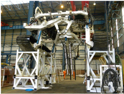
Figure 39 Typical ROV Jet trencher
