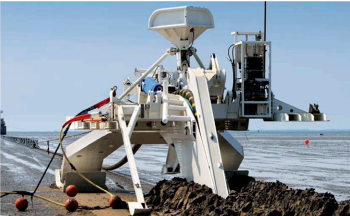
Figure 42 Sea Stallion cable plough
