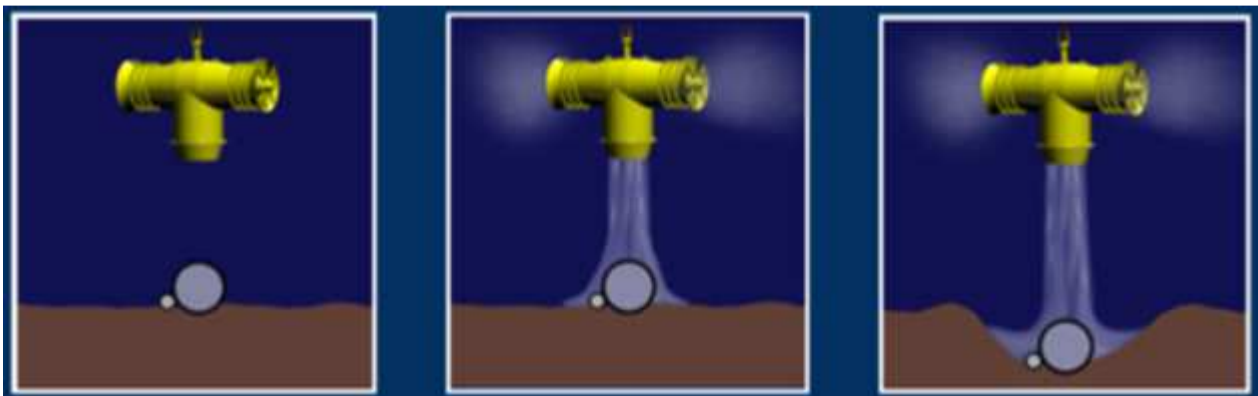
Figure 43 Mass flow excavation
