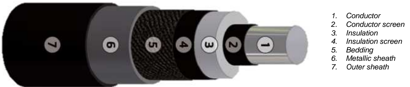
Figure 6 Typical HVAC 220 kV land export cable
