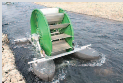
Barsha pump of aQysta at work
